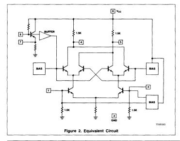
permissible oscillation frequency. If the required L.O. is beyond oscillation limits, or the system calls for an external L.O., the external signal can be injected at Pin 6 through a DC blocking capacitor. External L.O. should be at least  $200m/p_{p,p}$ .
