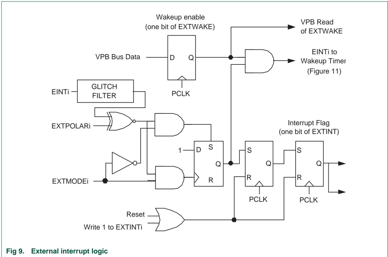
Fig 9. External interrupt logic
