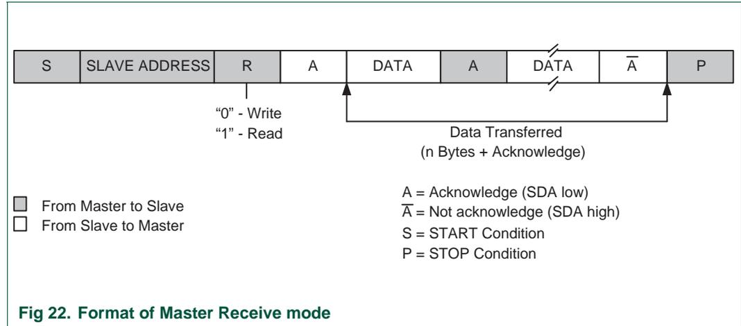
Fig 22. Format of Master Receive mode
