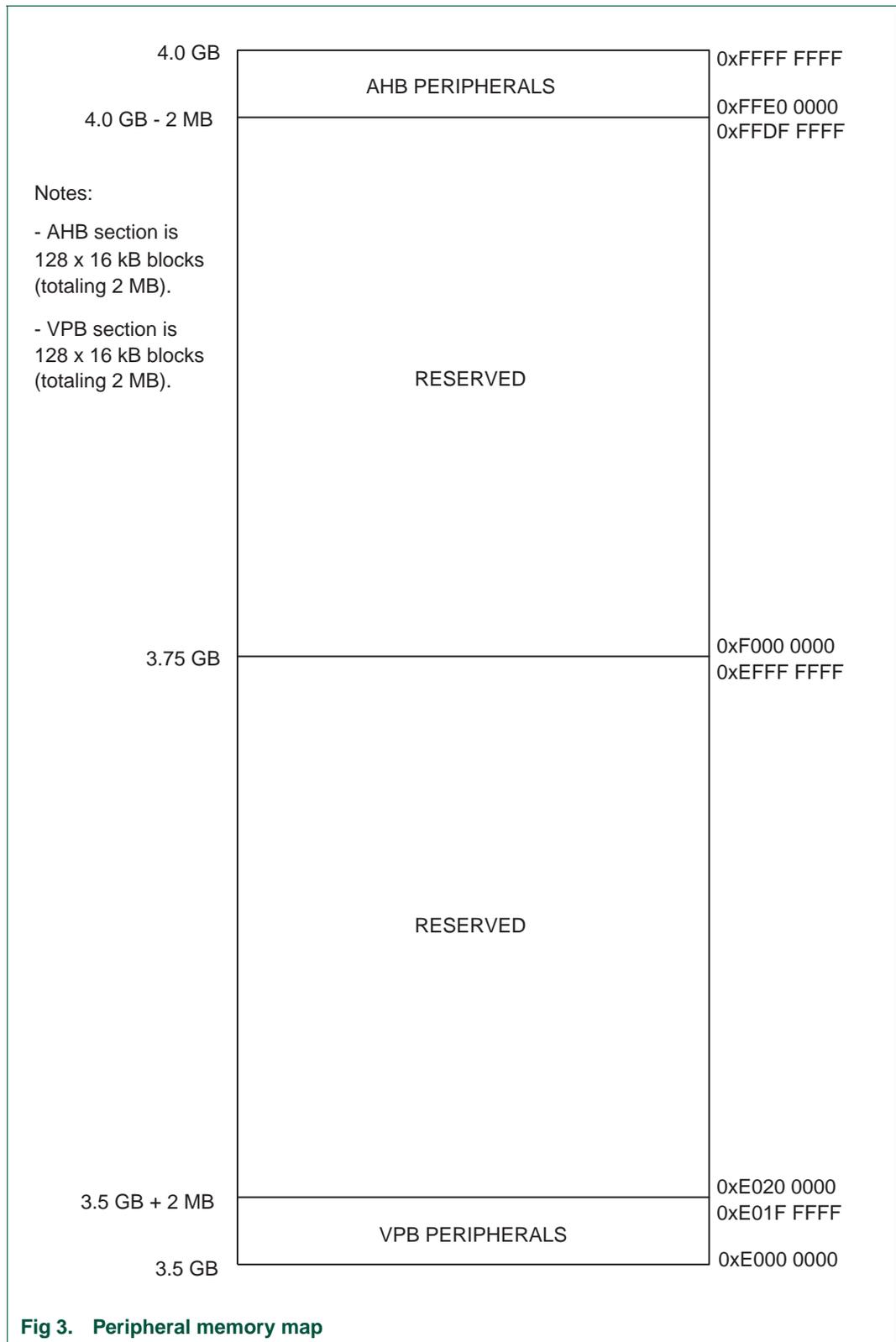
Figures 3 through 5 show different views of the peripheral address space. Both the AHB and VPB peripheral areas are 2 megabyte spaces which are divided up into 128 peripherals. Each peripheral space is 16 kilobytes in size. This allows simplifying the
