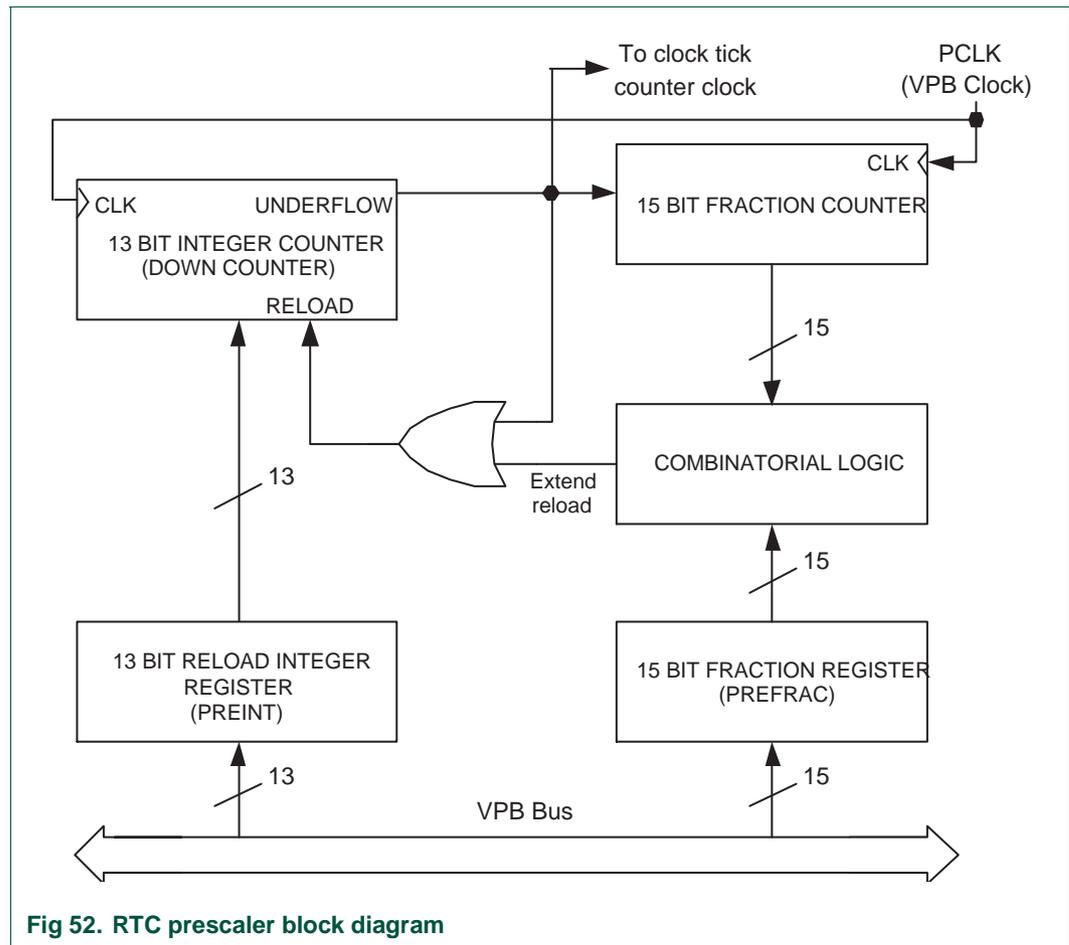
Fig 52. RTC prescaler block diagram
