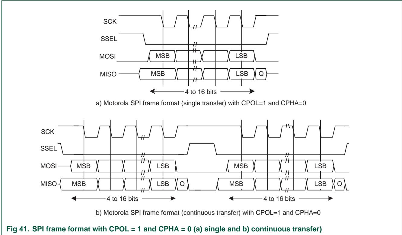
Fig 41. SPI frame format with CPOL = 1 and CPHA = 0 (a) single and b) continuous transfer)
