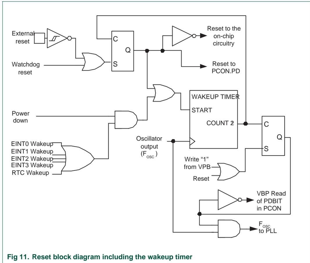
Fig 11. Reset block diagram including the wakeup timer
