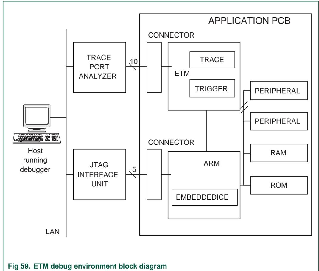
Fig 59. ETM debug environment block diagram
