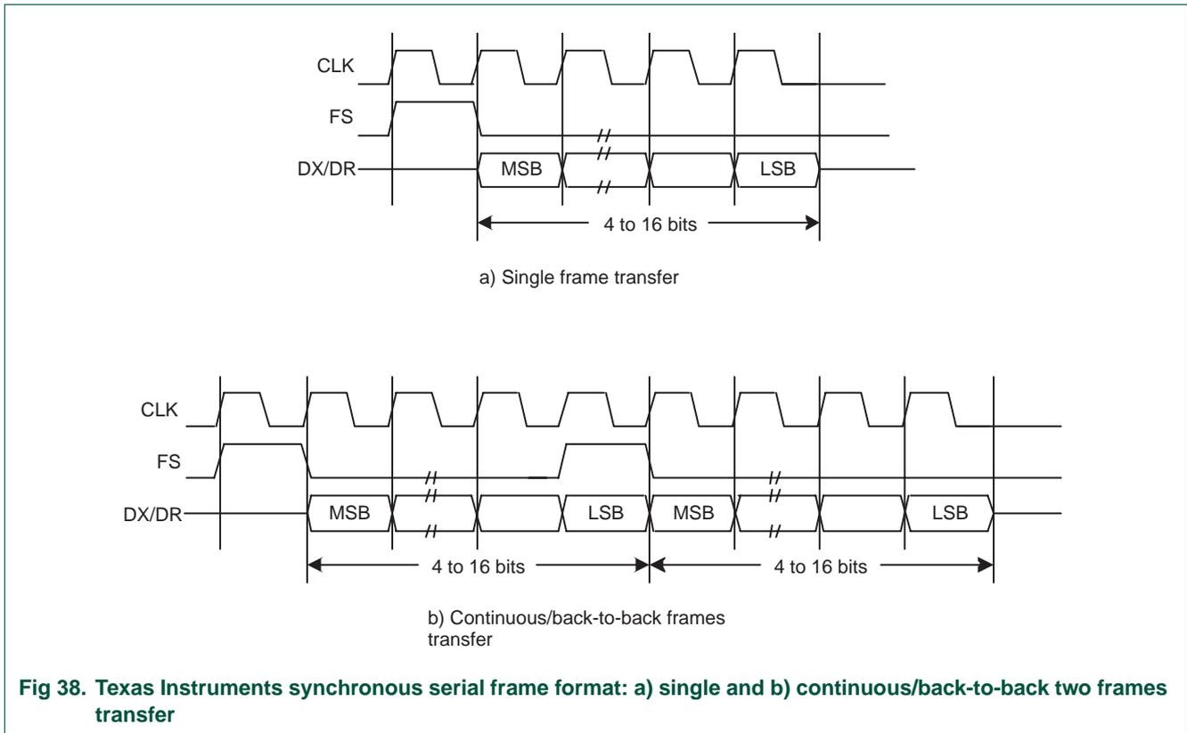
**Fig 38. Texas Instruments synchronous serial frame format: a) single and b) continuous/back-to-back two frames transfer**
