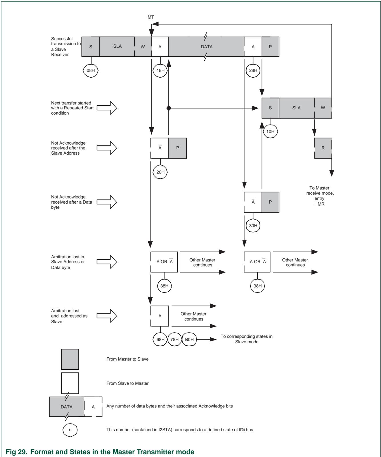
Fig 29. Format and States in the Master Transmitter mode
