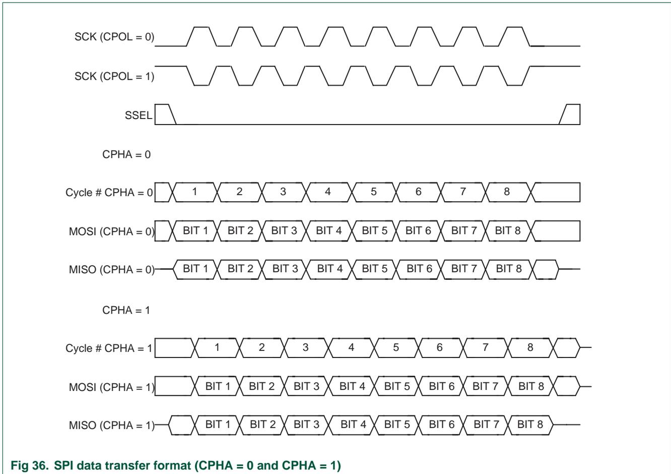
Fig 36. SPI data transfer format (CPHA = 0 and CPHA = 1)
