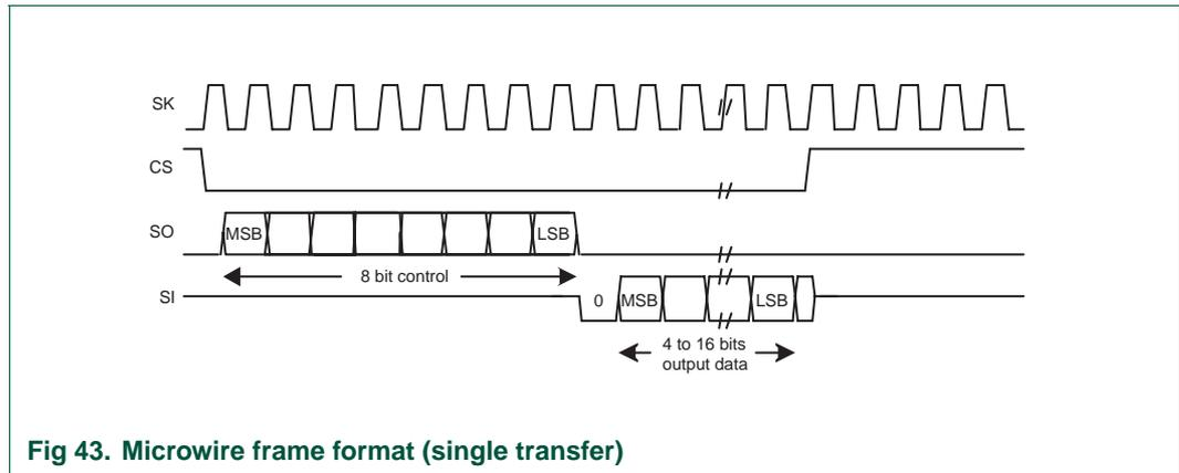
**Fig 43. Microwire frame format (single transfer)**
