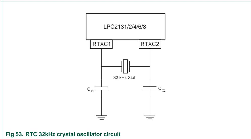
Fig 53. RTC 32kHz crystal oscillator circuit
