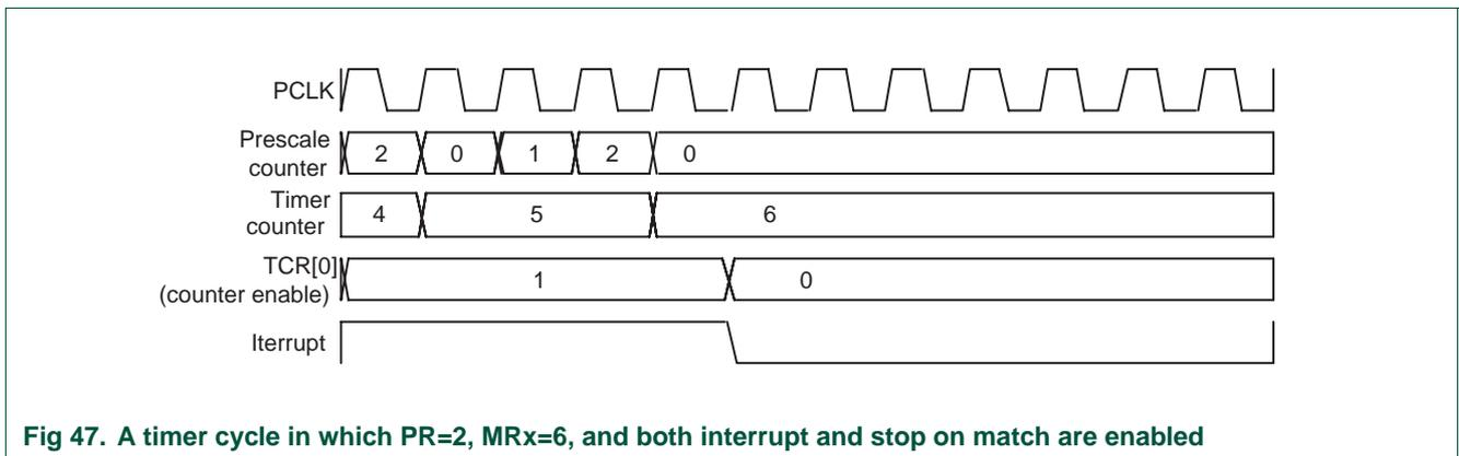
Fig 47. A timer cycle in which PR=2, MRx=6, and both interrupt and stop on match are enabled
