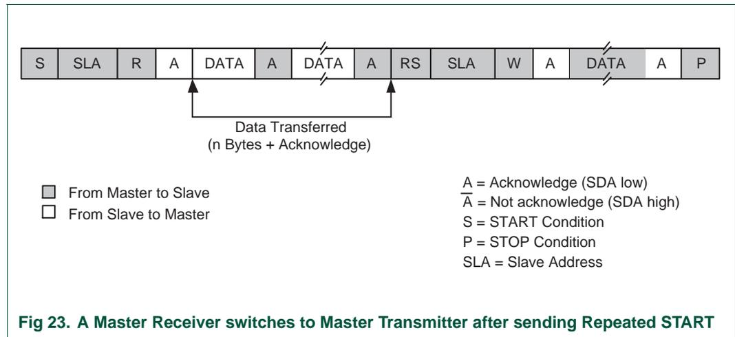
Fig 23. A Master Receiver switches to Master Transmitter after sending Repeated START
