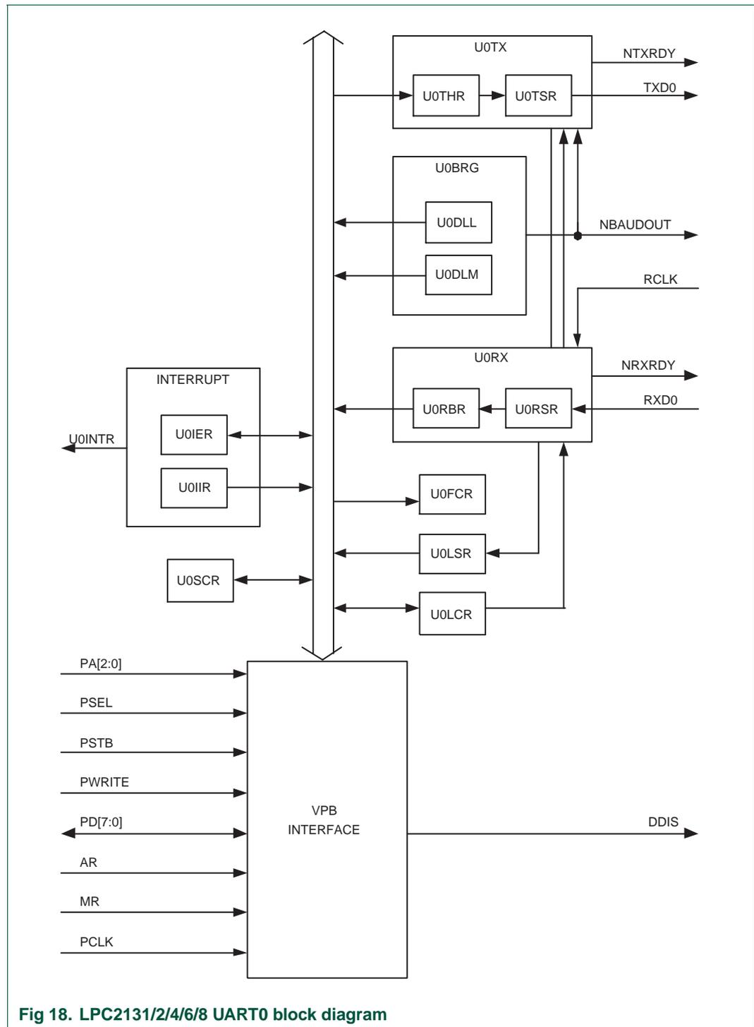
Fig 18. LPC2131/2/4/6/8 UART0 block diagram
