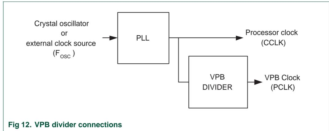
**Fig 12. VPB divider connections**
