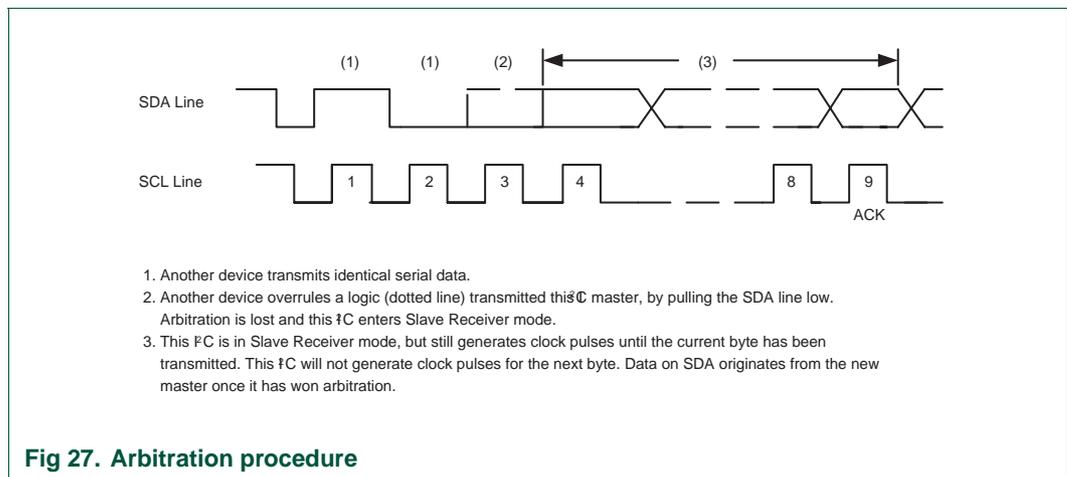
Fig 27. Arbitration procedure
