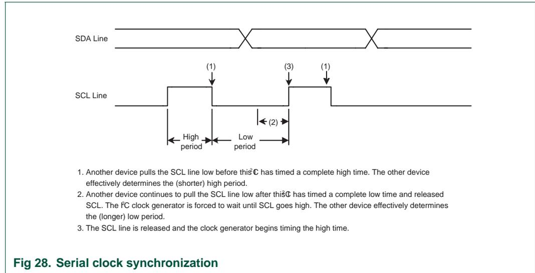
**Fig 28. Serial clock synchronization**
