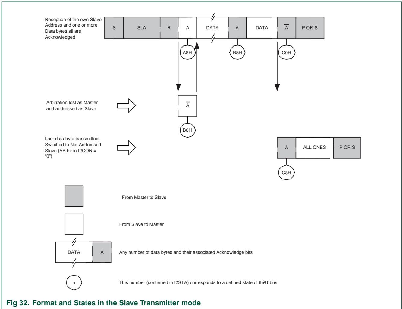
Fig 32. Format and States in the Slave Transmitter mode
