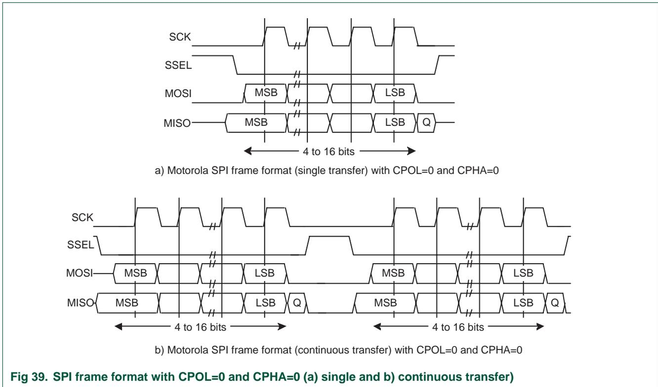
**Fig 39. SPI frame format with CPOL=0 and CPHA=0 (a) single and b) continuous transfer)**
