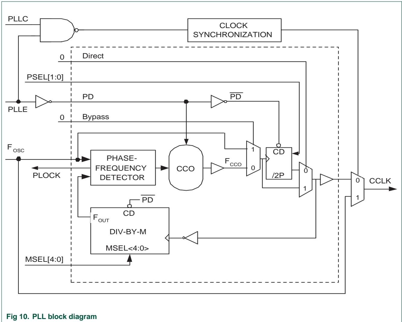
Fig 10. PLL block diagram
