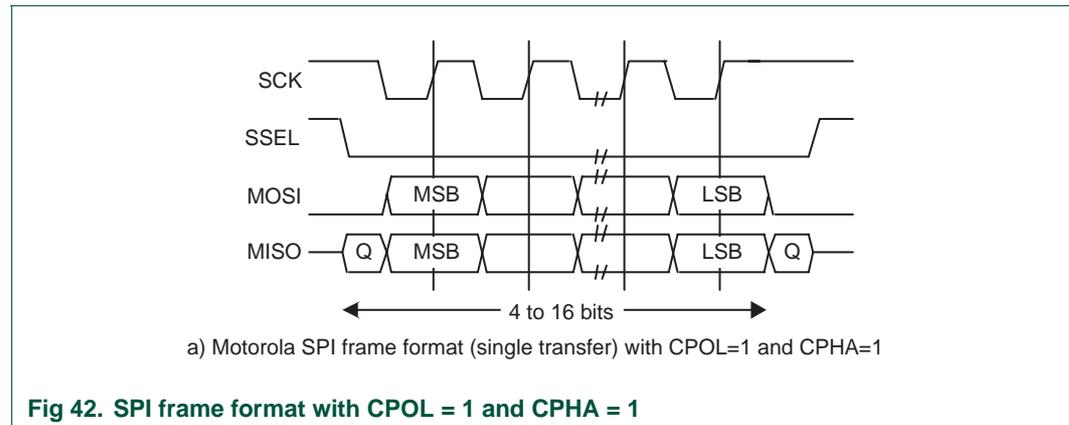
**Fig 42. SPI frame format with CPOL = 1 and CPHA = 1**
