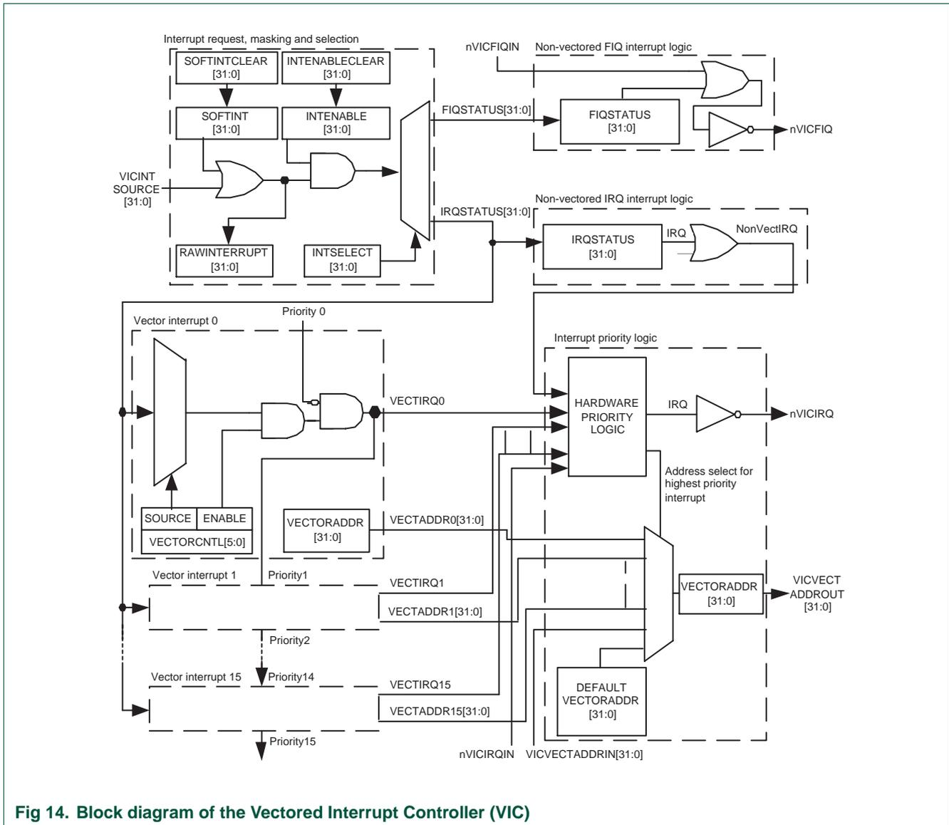
Fig 14. Block diagram of the Vectored Interrupt Controller (VIC)
