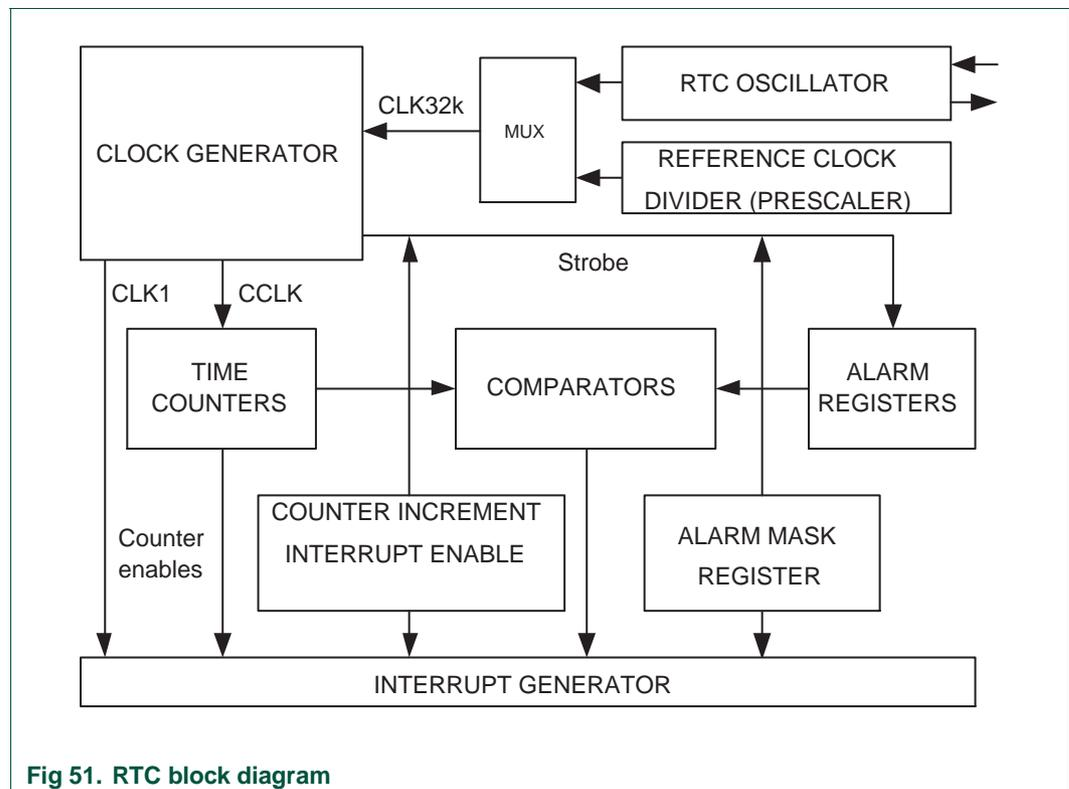
Fig 51. RTC block diagram
