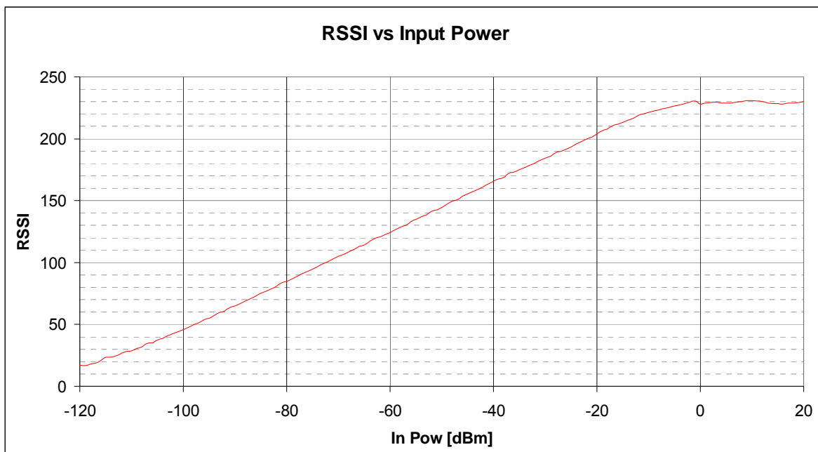
Figure 24. RSSI Value vs. Input Power
