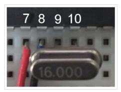
Here is a 16 MHz crystal used on a bread board Arduino connected to XTAL1 and XTAL2. The ATmega chip has to be told to use the external crystal and this is done by setting the CKSEL bits. A common mistake is to have the crystal correctly connected in the circuit but forget to tell the chip to use it.
