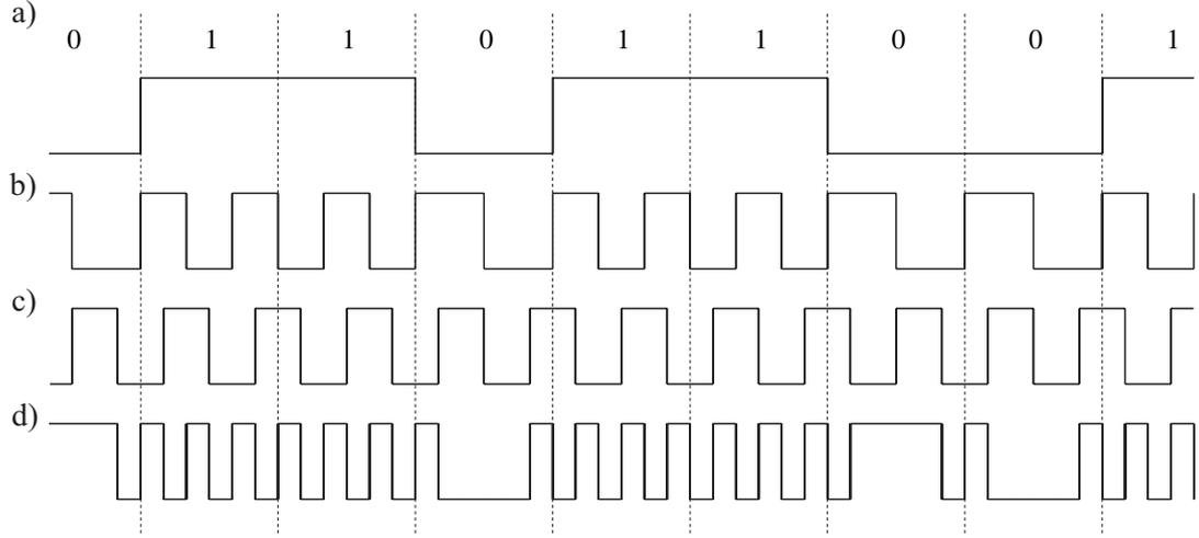
**Figure 3.** Illustration of the modulation: a) unmodulated pseudo-random sequence, b) Minimum-Shift-Keying (MSK)—Frequency-Modulation (FM) with sequence-conducted change of ranks, c) carrier with odd division for Phase-Modulation (PM), d) MSK-PM signal (XOR of b and c).
