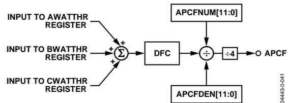
Figure 65. ADE7758 Active Power Frequency Output
