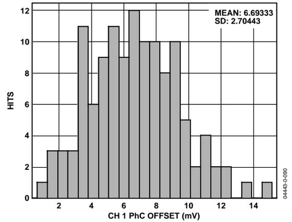
Figure 32. Phase C Channel 1 Offset Distribution
