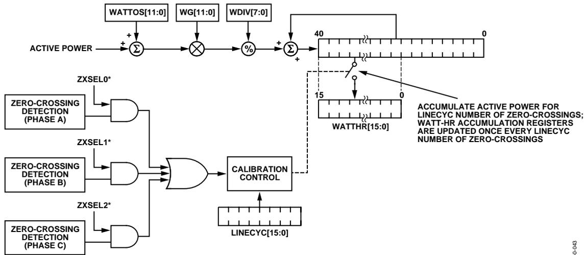
\*ZXSEL[0:2] ARE BITS 3 TO 5 IN THE LCYCMODE REGISTER
