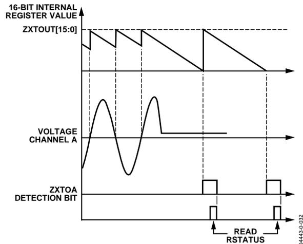
Figure 50. Zero-Crossing Timeout Detection
