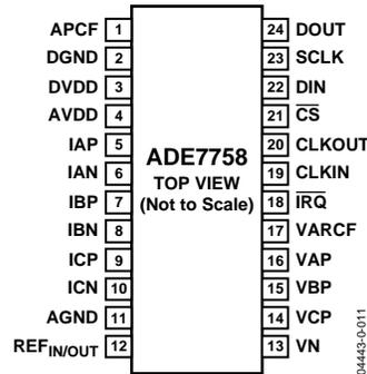
Figure 35. Pin Configuration
