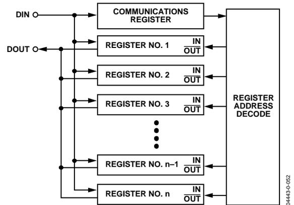
Figure 85. Addressing ADE7758 Registers via the Communications Register
