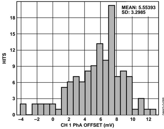
Figure 30. Phase A Channel 1 Offset Distribution
