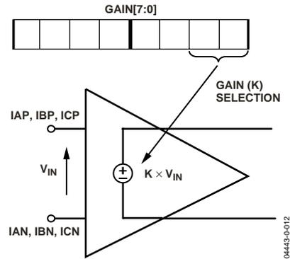
Figure 36. PGA in Current Channel
