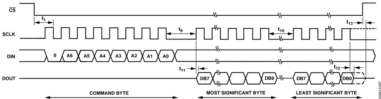
Figure 90. Serial Interface Read Timing Diagram
