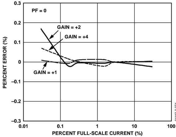
Figure 18. Reactive Energy Error as a Percentage of Reading over Gain with Internal Reference and Integrator Off
