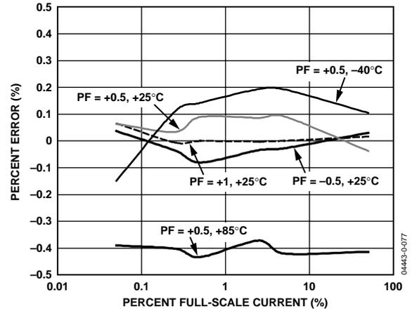
Figure 21. Active Energy Error as a Percentage of Reading (Gain = +4) over Power Factor with Internal Reference and Integrator On
