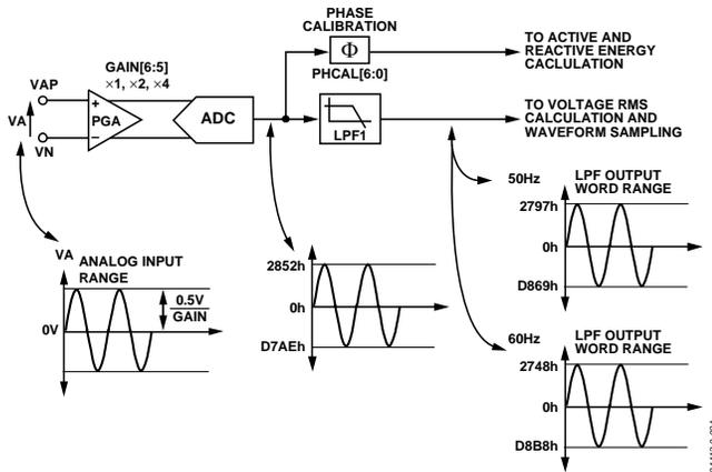
Figure 47. ADC and Signal Processing in Voltage Channel
