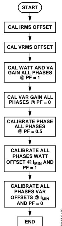
Figure 77. Calibration Using Line Accumulation
