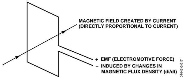
Figure 40. Principle of a di/dt Current Sensor
