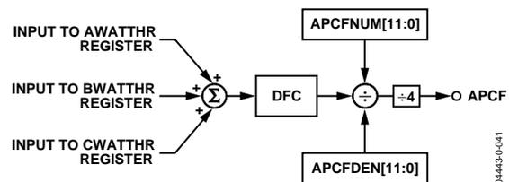
*Figure 65. ADE7758 Active Power Frequency Output*
