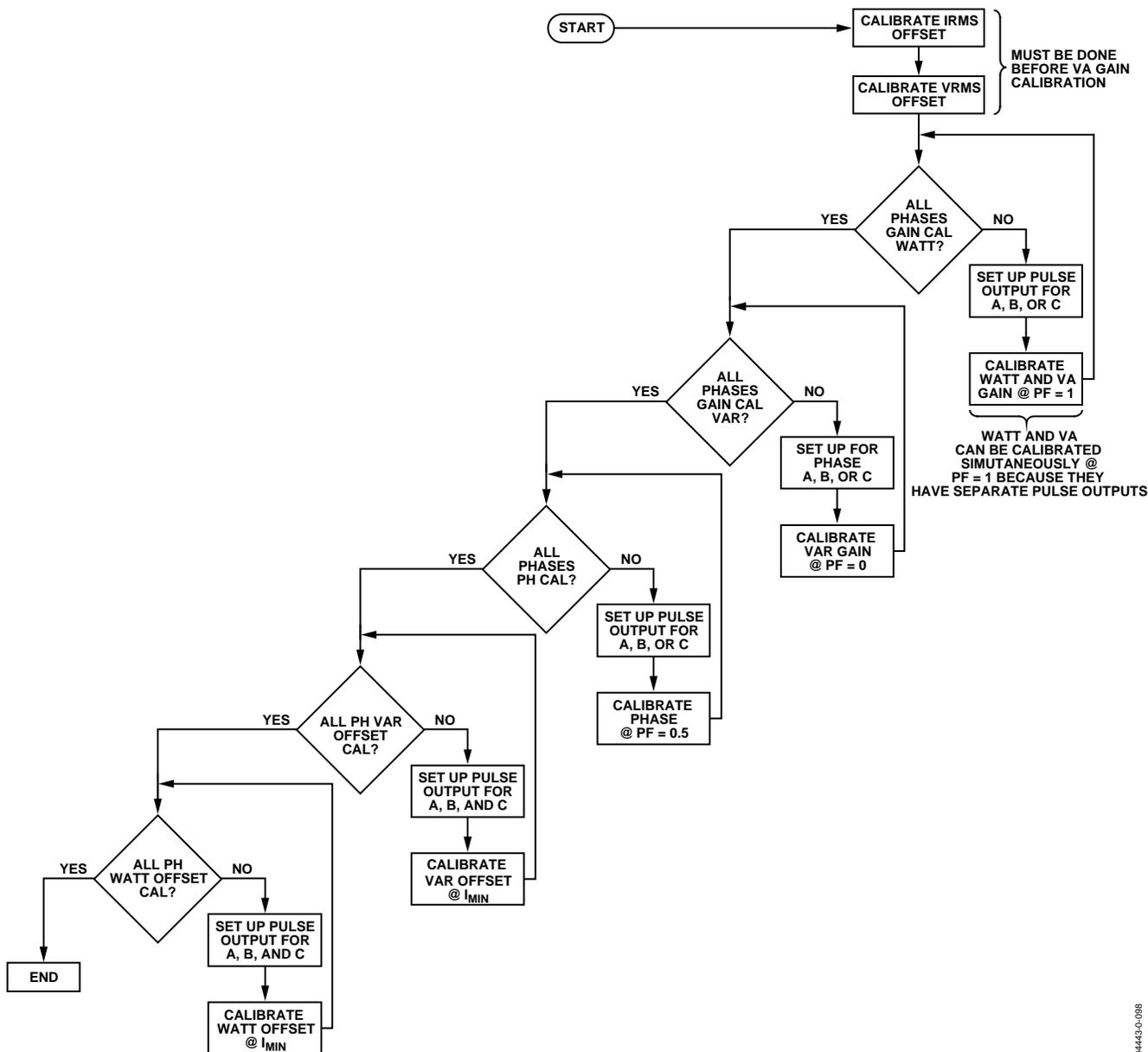
Figure 73. Calibration Using Pulse Output
