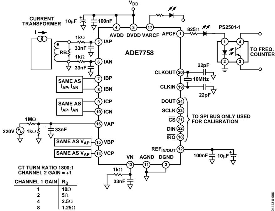
Figure 33. Test Circuit for Integrator Off
