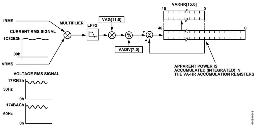
Figure 72. ADE7758 Apparent Energy Accumulation
