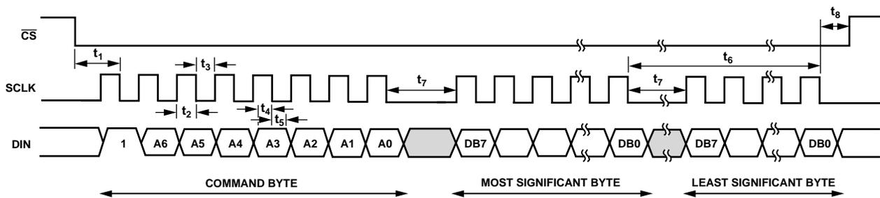
Figure 88. Serial Interface Write Timing Diagram
