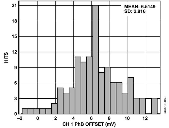
Figure 31. Phase B Channel 1 Offset Distribution
