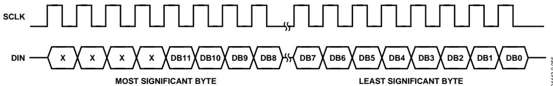
Figure 89. 12-Bit Serial Write Operation
