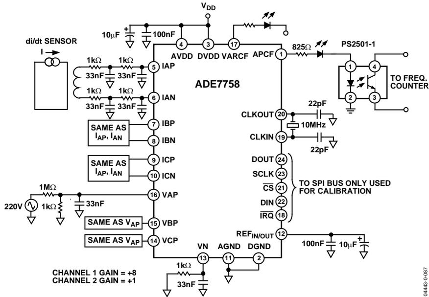
Figure 34. Test Circuit for Integrator On
