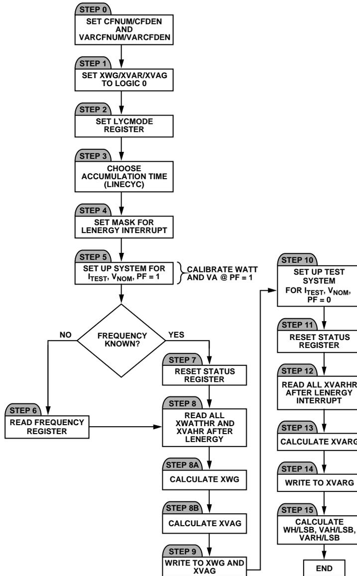
Figure 78. Gain Calibration Using Line Accumulation
