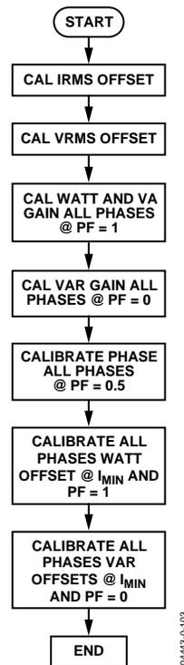
Figure 77. Calibration Using Line Accumulation
