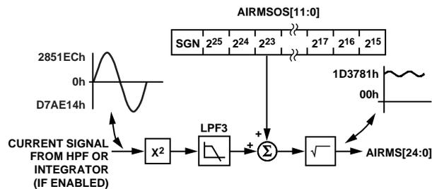
Figure 59. Current RMS Signal Processing
