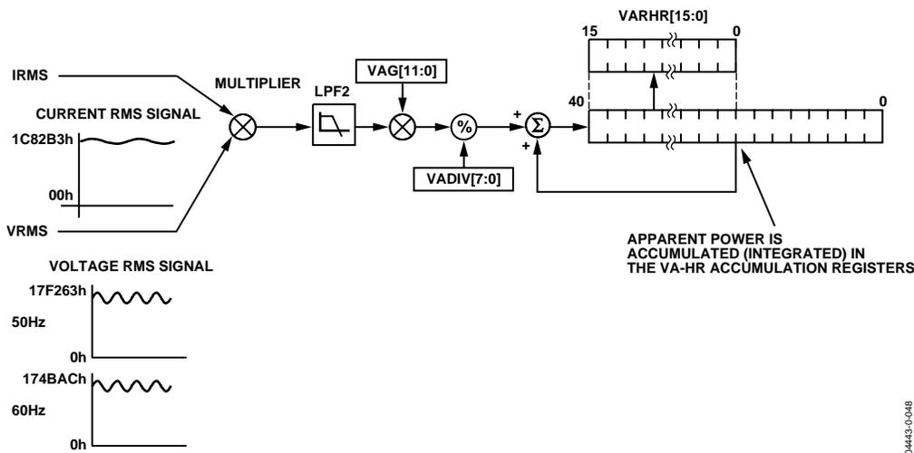
Figure 72. ADE7758 Apparent Energy Accumulation
