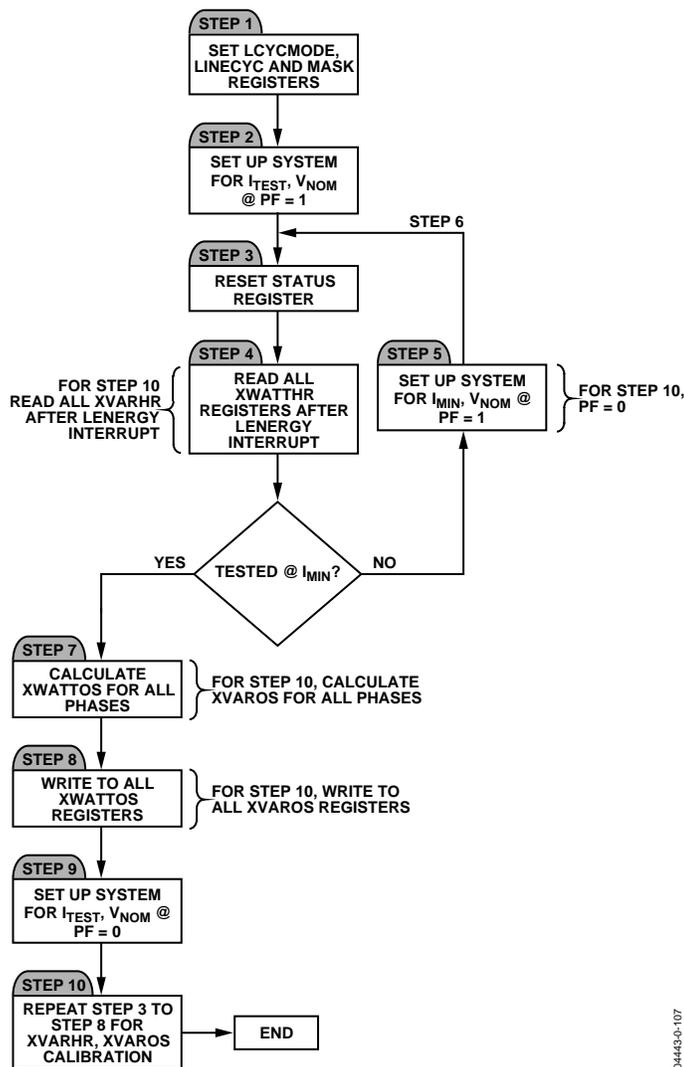
Figure 80. Power Offset Calibration Using Line Accumulation
