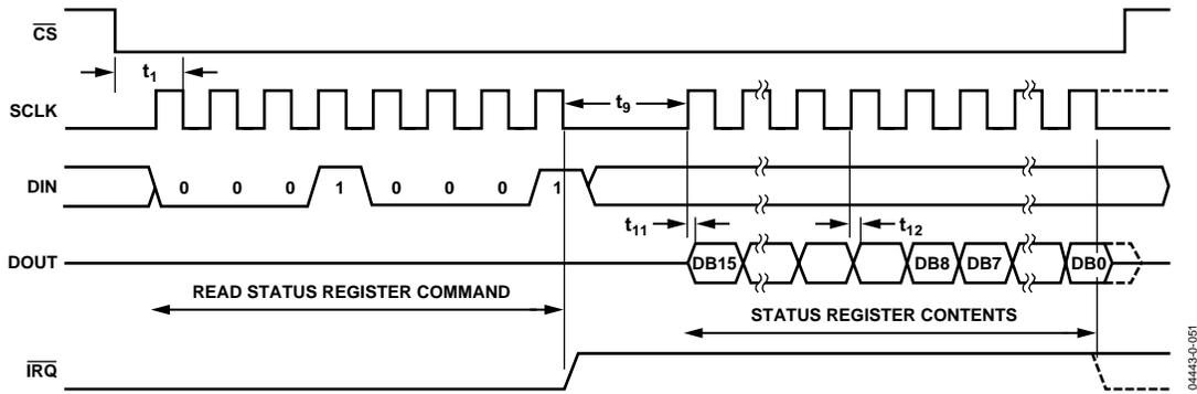
Figure 84. ADE7758 Interrupt Timing
