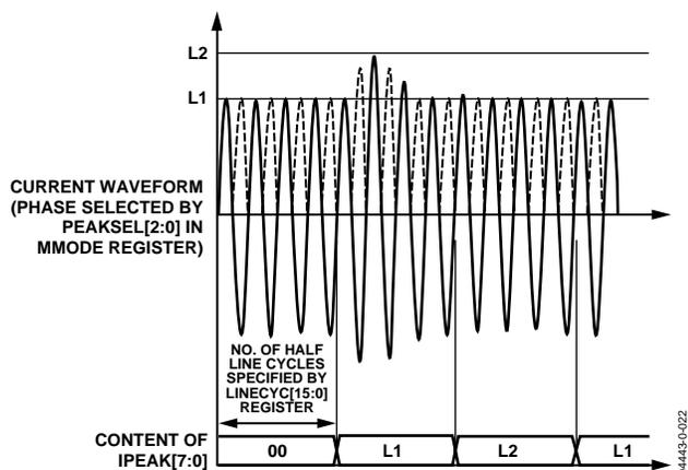
Figure 45. Peak Current Detection Using the IPEAK Register
