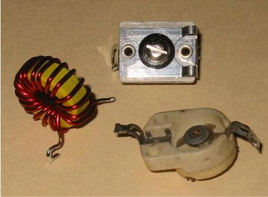
The inductor is our "standard, L2" used for many of these measurements. The upper trimmer is the mica compression measured in case 14 while the lower capacitor is the rotary ceramic part measured in case 15.
