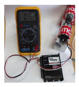
Figure 8 Using an ESCON as a rectifier.
