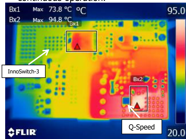
Figure 112 – 130 VDC 2.5A Full Load. Temperature of InnoSwitch3-AQ: 73.8 °C. Temperature of SR FET: 94.8 °C. Ambient Temperature: 27.3 °C.
