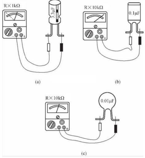
Figure12. (a) Normal; (b) Breakdown; (c) Failure
