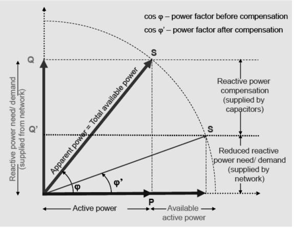
Figure11. Reactive Power Compensation Supplied by Capacitors
