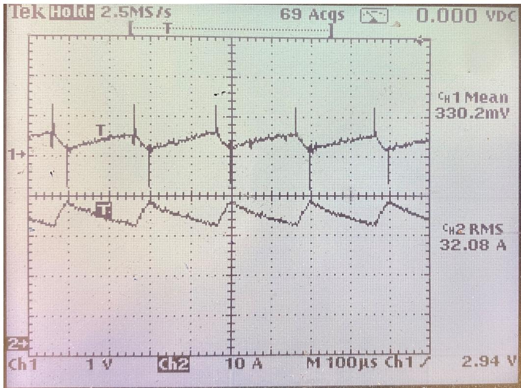
CH 1: Messignal Strom LEM Wandler ( $2,5 \text{ V} = 0 \text{ A} / 0 \text{ V} = 36 \text{ A} / 5 \text{ V} = -36 \text{ A}$ )
