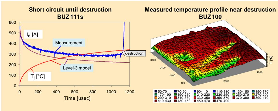
**Fig. 12:** At very high junction temperatures, larger temperature deviations occur due to influences not taken into account in the model. On the right is a high-speed thermograph photo of the chip surface close to the destruction point.
