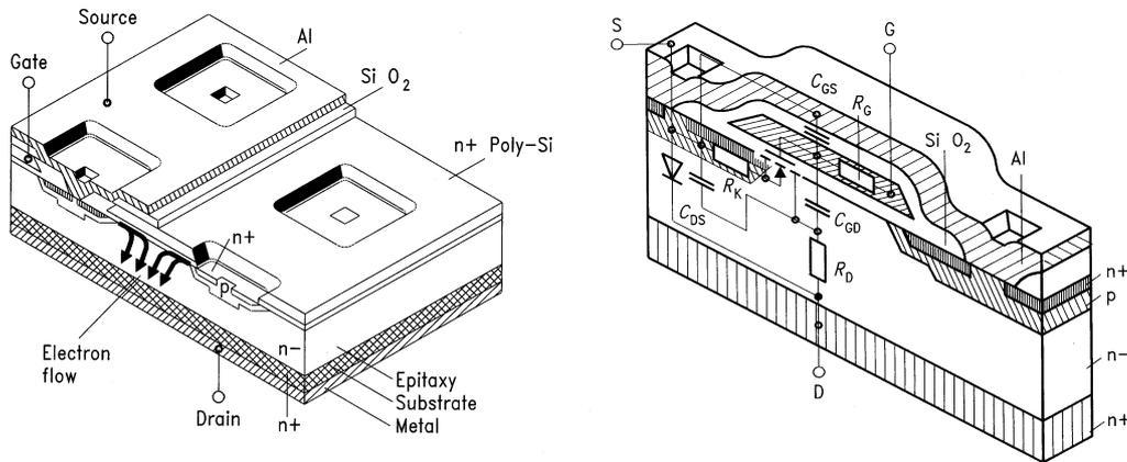
**Fig. 6:** Structure of a power MOSFET (DMOS) with the parasitic elements important for the component behavior
