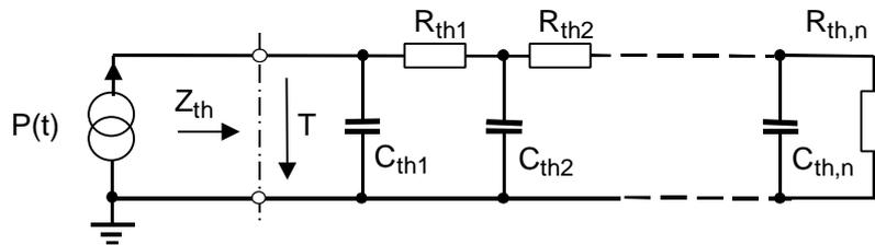
**Fig. 1:** Electrical transmission line equivalent circuit diagram for modeling heat conduction properties; the physical variables are specified in their thermal equivalents.
