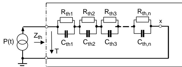
**Fig. 3:** The most frequently used thermal equivalent circuit diagram is mathematically very simple to use but as a purely formal description has no relation to the real physical structure.
