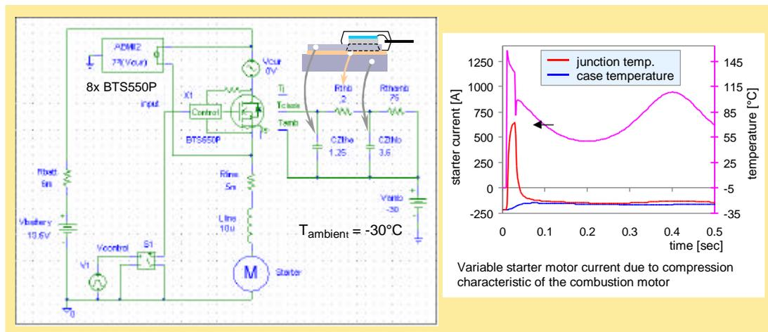
**Fig. 15:** Dynamic temperature modeling forms the basis for Smart Power simulation models. The actuation of a car starter by means of several high current PROFETs is illustrated.
