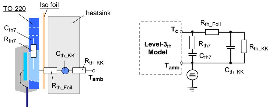
**Fig. 13:** A practical example of a first order thermal equivalent circuit diagram for a transistor with heat sink.
