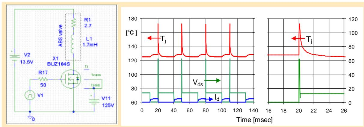
**Fig. 14:** Simulation of the junction temperature in periodic avalanche operation
