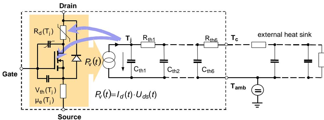
**Fig. 8:** Principle circuit diagram of a model with interactive coupling of electrical and thermal component description (“Level-3<sub>th</sub>” model).
