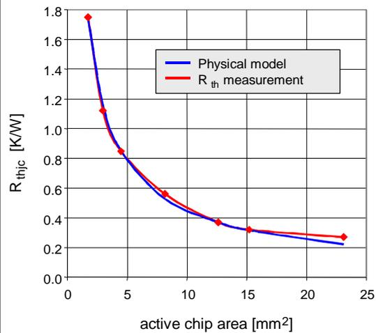
**Fig. 5:** Comparison of the thermal resistance calculated according to figure 2 with measured values for different chip surfaces in a TO-220 package
