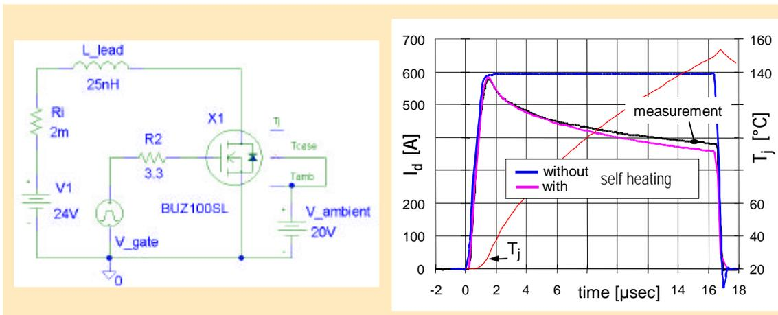
Fig. 10: Result of a short-circuit simulation with and without consideration of the inherent self-heating
