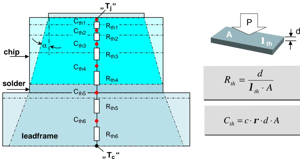
**Fig. 2:** For simple structures, the thermal equivalent elements can be determined directly from the physical structure. For the sake of clarity, the actual thickness relationships are not shown to scale.
