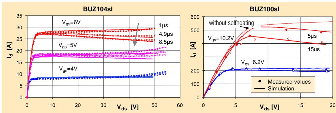
**Fig. 11:** The current drop due to inherent heating in the output characteristic becomes noticeable already after very short pulses.
