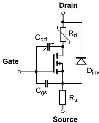
**Fig. 7:** The circuit diagram of a DMOS model shows the principals and reflects the structural elements of figure 6
