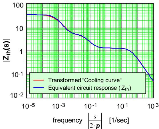
**Fig. 4:** A  $Z_{thj}(s)$  curve determined from a cooling curve and an adapted line equivalent circuit diagram (here: SMD package on board).
