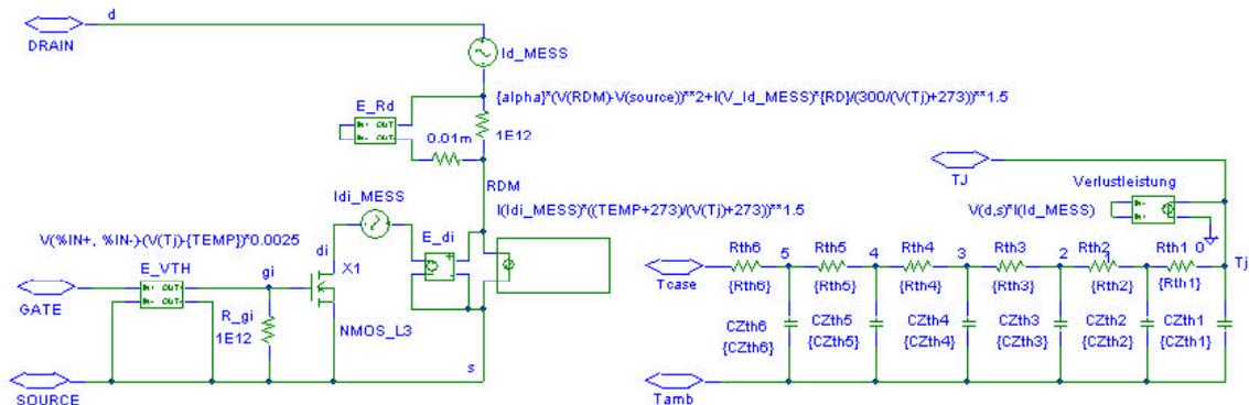
**Fig. 9:** MOSFET model created in PSPICE with dynamically temperature-dependent parameters
