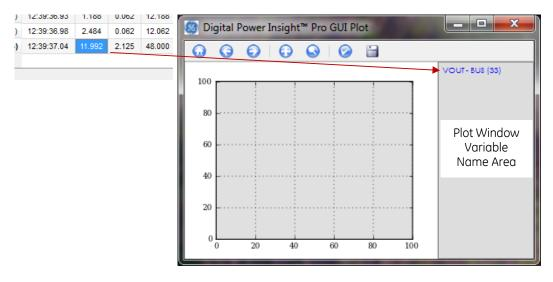
To select multiple module variables for plotting, repeat the process of selecting and dragging module variables to the Plot Window Variable Name Display area. Note that multiple module names can be selected in the Module Status window by using the <CTRL>+Click (for a sequence of names) or <SHIFT>+Click to select an area of module names for plotting. Examples of the Module status window when multiple module names are selected are shown below.
