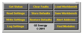
**Get Status**: Used to read a single set of parameter and status values from the selected module (module can be selected by clicking on one of the **Selected Module** buttons at the bottom of each column in the Module Settings area). When this command is activated by clicking on the button, the module status is refreshed in the tool, and the last display of readings is maintained.
