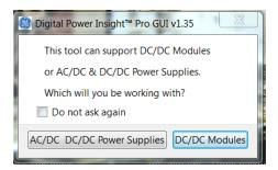
This screen asks the user to select the product family that is going to be connected so the tool can configure the appropriate set of features.. If the **Do not ask again** box is checked, the Pro\_GUI tool will start with settings configured in the previous session. The user can reconfigure the product family setting as shown below.
