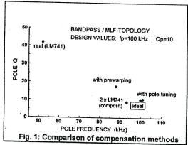
into consideration - as well as other error sources, e.g. deviations from calculated component values, load impedances or parasitic capacitances and inductances. By applying this technique the accuracy of the filter response is improved considerably. As illustrated in Fig. 1 where the pole parameters  $Q_P$  resp.  $f_P$  are compared for different compensation methods it is possible to shift the dominant pole very close to the ideal position.
