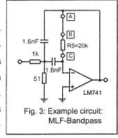
As mentioned earlier, bandpass optimization requires adjusting the loop gain at  $f_P$ . Note that the MLF-topology is one of the exceptional cases where the OA is *not* used as a controlled source with local feedback. Therefore, the *ideal* loop gain of the filter approaches infinity, and only one sub-loop (in this case branch R5) may be considered.
