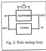
However, it is the primary aim of the procedure to shift the *pole* of the filter towards the ideal position! Because, on the other hand, the pole location is directly related to the circuits *loop gain* at pole frequency  $f_P$ , the block NETWORK must contain, therefore, the filter circuit with an *open* feedback loop. Thus, the basic idea of the method is to set the filter's *loop gain* at  $f_Z = f_P$  to its proper value (in magnitude and phase), thereby correcting the pole parameters.
