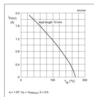
Fig.2 Maximum permissible average forward current as a function of tie-point temperature (including losses due to reverse leakage).
