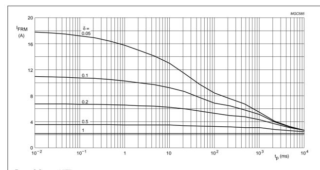
$$\begin{split} &T_{tp}=55^{\circ}\text{C}; \ R_{th \ j\text{-}tp}=46 \ \text{K/W}. \\ &V_{RRMmax} \ \text{during 1} - \delta; \ \text{curves include derating for T}_{j \ max} \ \text{at V}_{RRM} = 1000 \ \text{V}. \end{split}$$
