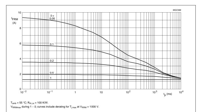
Fig.5 Maximum repetitive peak forward current as a function of pulse time (square pulse) and duty factor.
