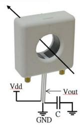
Capacitor C(0.01uF~0.1uF) is recommend to be connected between Vout and GND to reduce output noise.
