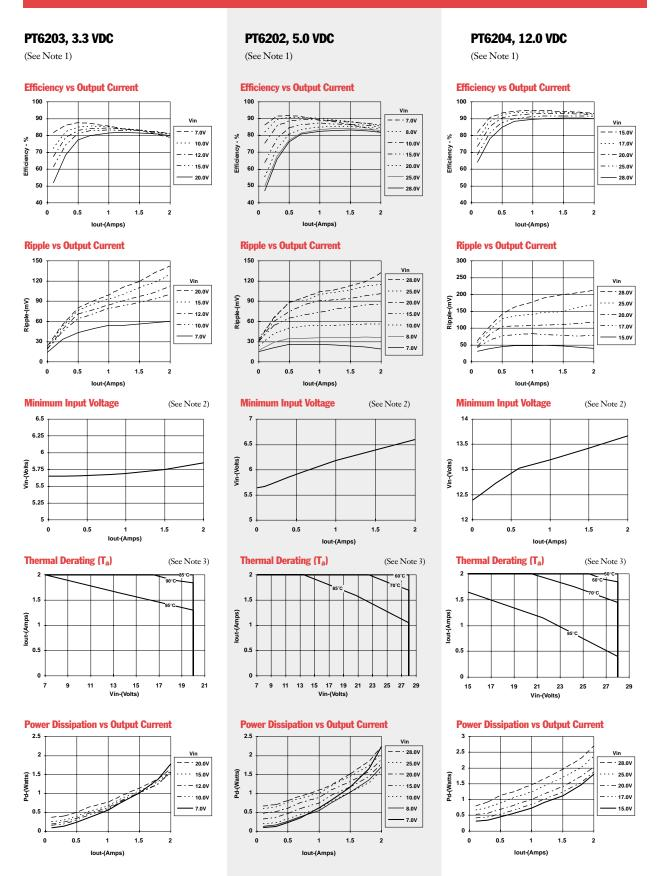
Note 1: All data listed in the above graphs, except for derating data, has been developed from actual products tested at 25°C. This data is considered typical data for the ISR.
