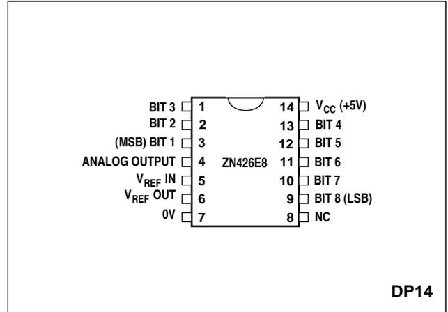
Fig.1 Pin connections (not to scale) - top view
