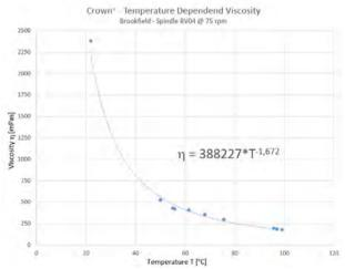
Figure 2. Viscosity characteristics of one target dental material
