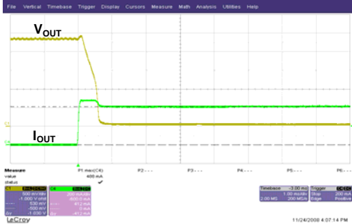
Current Limit ( V_{OUT} vs. I_{OUT} )
