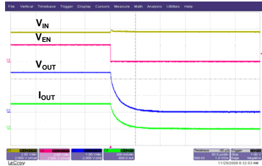
Enable OFF Sequence ( R_L=8\Omega ) V_{EN}=2V to 0V
