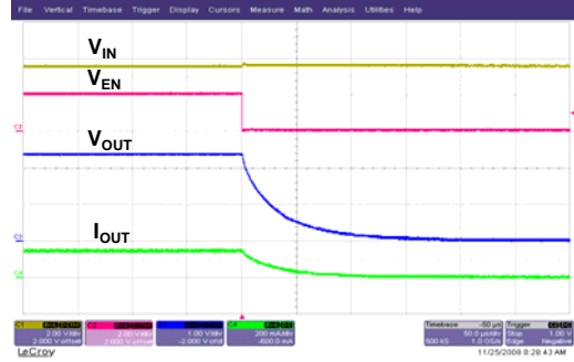
Enable OFF Sequence ( R_L=16\Omega ) V_{EN}=2V to 0V
