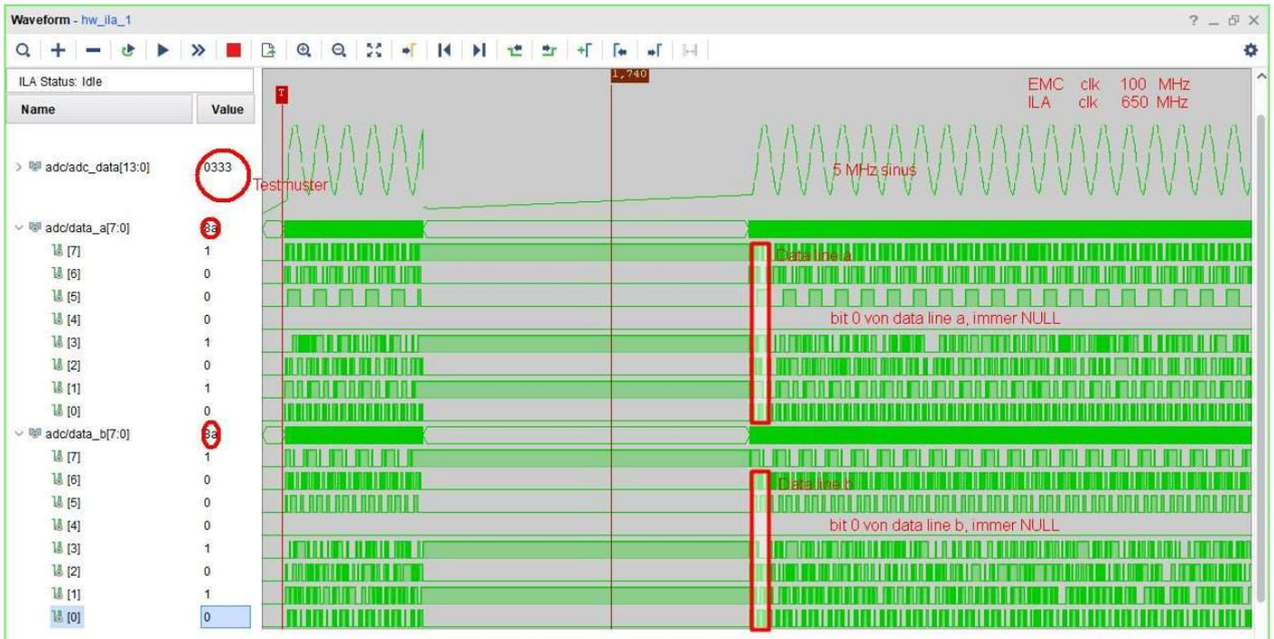
Delay DCO clk (400 MHz): 0 counts, Data (400 MHz): 256 counts, Frame clk (100 MHz): 511 counts
