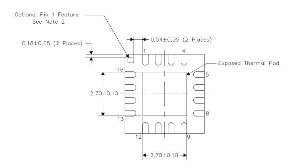
Bottom View Exposed Thermal Pad Dimensions
