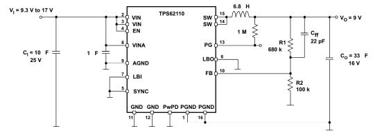
A. For an output voltage greater than 5 V, an output capacitor of 33 µF minimum is required for stability.
