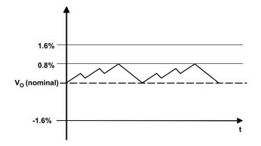
Figure 18. Power Save Mode Output Voltage Thresholds
