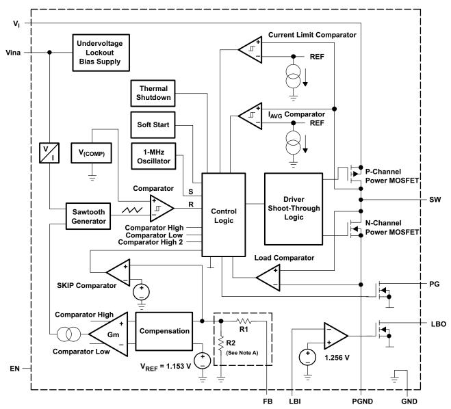
A. For the adjustable version (TPS62110), the internal feedback divider is disabled and the FB pin is directly connected to the internal GM amplifier.
