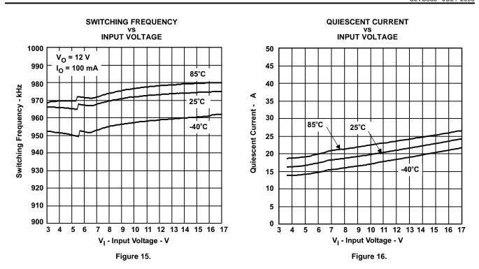
The graphs were generated using the EVM with the setup according to Figure 17 unless otherwise noted. The output voltage divider was adjusted according to Table 4. Graphs for an output voltage of 5 V and 3.3 V were generated using TPS62111 and TPS62112 with R1 = 0  $\Omega$  and R2 = open.
