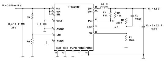
A. For an output voltage lower than 2.5 V, an output capacitor of 33  $\mu$ F or greater is recommended to improve load transient.
