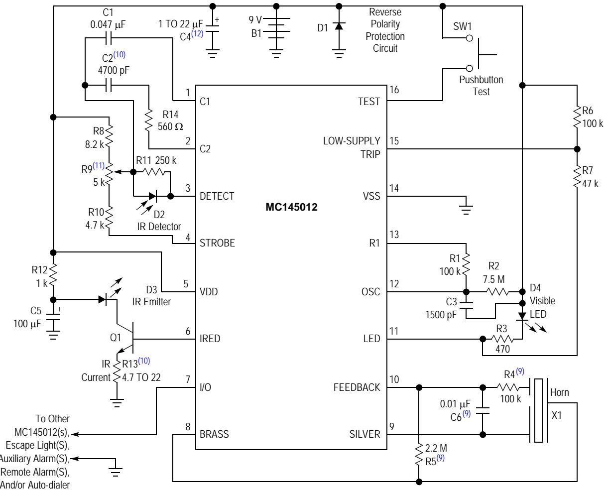
9. Values for R4, R5, and C6 may differ depending on type of piezoelectric horn used.
