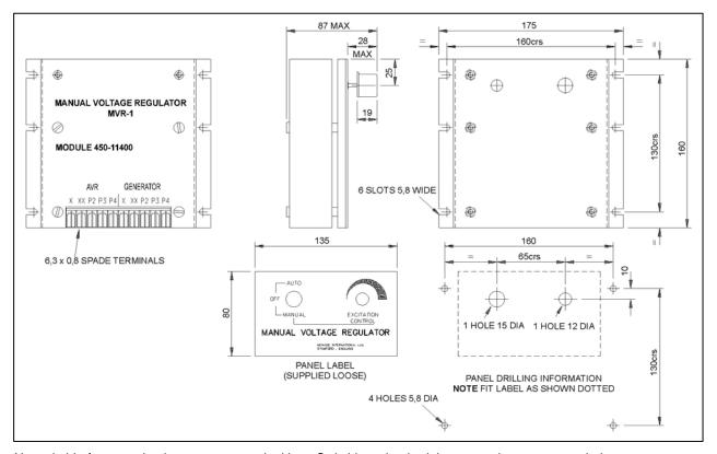
Not suitable for mounting in generator terminal box. Switchboard or bedplate mounting recommended.
