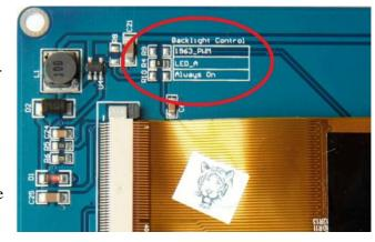
used to short the nearby pair of solder pads marked "1963-PWM". The PicoMite can then control the brightness via the SSD1963 controller using the BACKLIGHT command.
