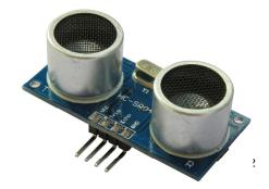
This device can be found on eBay for about \$4 and it will measure the distance to a target from 3cm to 3m. It works by sending an ultrasonic sound pulse and measuring the time it takes for the echo to be returned.
