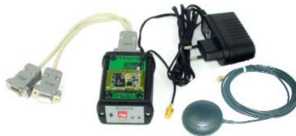
Figure 17: JP7-T Evaluation board
