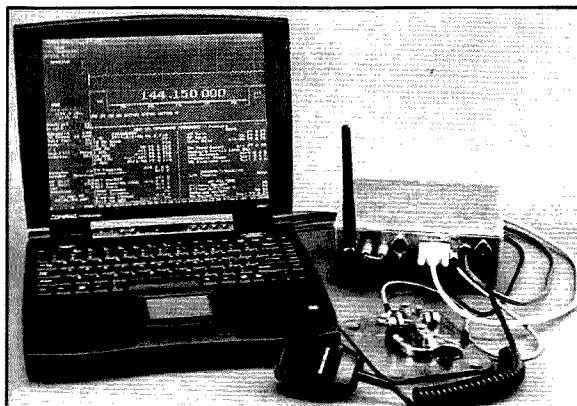
A complete QRP rig for 2-meters, the DSP-10, is built around a minimal amount of hardware and the software running in the laptop PC. Along with the RF hardware in the die-cast box is an Analog Devices EZ-KIT Lite that serves as the last IF and audio portions of the transceiver. See page 11.27 for more information.
