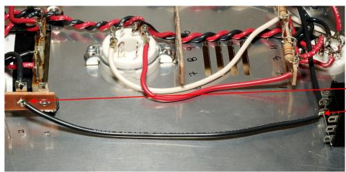
() Cut a piece of black wire 6-1/2" (167mm) long and strip both ends 1/4" (6mm). Attach one end to terminal 12L and solder. Attach the other end to the inboard terminal of the headphone jack that is closest to the chassis plate, and solder.
