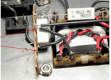
( ) Cut a piece of black wire 2" (50mm) long and strip both ends 1/4" (6mm) Attach one end to terminal 14U Attach the other end to terminal 12U.
