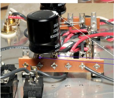
() Bend the lugs of a second 220uF 250V electrolytic capacitor at 90 degrees. Insert the lug by the striped side of the capacitor into terminal 14U. Insert the non striped side lead into terminal 15U. Double check orientation and solder.
