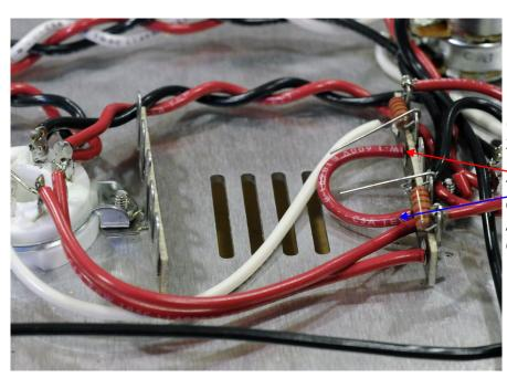
() Cut a piece of red wire 2" (50mm) long and strip both ends 1/4" (6mm). Attach one end to terminal 2L and solder. Attach the other end to terminal 4L and solder. Also solder 2U and 4U and trim any excess leads.
