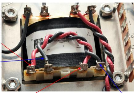
() At the other end of the twisted pair attach the red wire to power transformer terminal 9 and the black wire to power transformer terminal 10.
