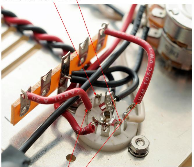
() Cut a 1-1/2" (37mm) piece of red wire and strip both ends 1/4" (6mm). Attach and solder one end to A6. Attach the other end to terminal 1U.
