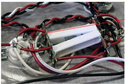
() Cut a 5-1/2" (137mm) white wire and strip both ends 1/4". Attach one end to terminal 10L and solder. Route the wire around the terminal strip as shown. Attach the other end to the inboard Tip terminal of the TRS phone jack.
