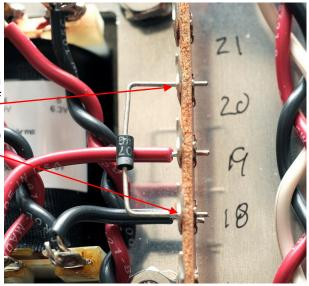
( ) Bend the leads of the second UF4007 rectifier with leads 1/2"(12mm) from the rectifier body. Line the rectifier body up over the first one on the same side of terminal strip, with the black end attached and soldered to terminal 18L and the banded end attached to terminal 21L. Trim excess leads from 18L.
