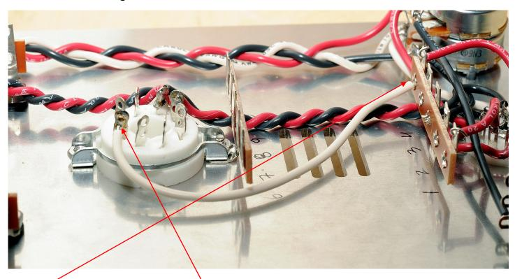
() Cut a 5" (125mm) piece of white wire. Strip both ends 1/4" (6mm). Attach and solder one end to 5L. Attach and solder the other end to B4.
