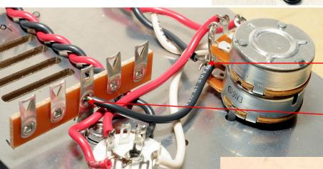
( ) Cut a 2-1/2" (62mm) piece of black wire and strip both ends 1/4" (6mm).
