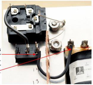
() Cut a 3-1/2" (88mm) piece of black wire and strip both ends 1/4". Attach and solder one end to terminal N of the power entry jack. Attach and solder the other end to terminal 2 of the power transformer.
