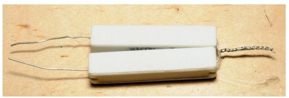
( ) Trim all but 1/4" (6mm) from the twisted end of the resistors and insert the trimmed end into terminal 3U. Insert the free lead of one resistor through terminal7L. Insert the other free resistor lead through terminal 9L. Solder 3U, 7L, 9L and trim the excess leads.
