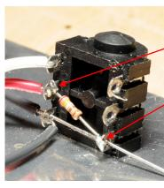
() Attach one end of a 2.49K ohm resistor to the inboard Ring terminal of the headphone jack.
