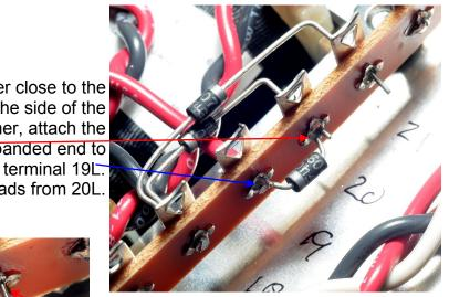
() Bend the leads of a fourth UF4007 rectifier 3/8" (9mm) from the rectifier body. With the rectifier located on the side of the terminal strip away from the power transformer, attach the black end to 19L and attach the banded end to terminal 21L. Solder 19L, 21L and trim excess leads.
