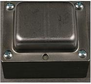
( ) Slip a round #8 lockwasher over one 1-3/4" screw and place that screw in the hole nearest the safety ground. Place three more #8 by 1-3/4"
