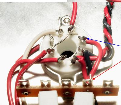
( ) Cut a 1-1/2" (37mm) red wire and strip both ends 1/4". Attach one end to terminal 9U and attach the other end to B6, Solder B6
