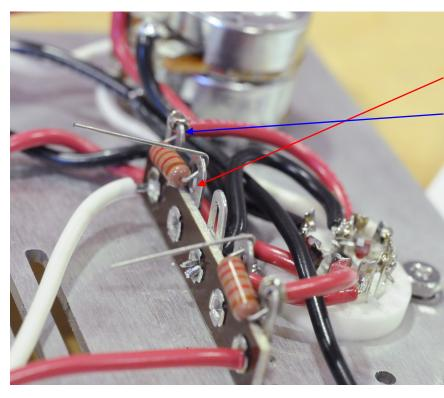
( ) Attach one end of an 22.1K ohm 1W resistor to 4U. Attach the other end to 5U. Solder 5U.
