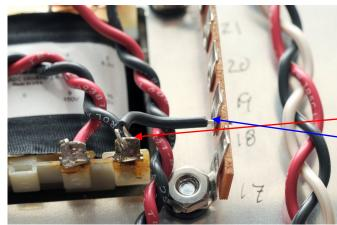
() Cut a 1-1/2" (37mm) piece of black wire and strip both ends back 1/4" (6mm). Attach and solder one end to power transformer terminal 10. Attach the other end to terminal 18L.
