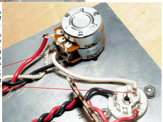
( ) Cut a 2-3/4" (70mm) piece of red wire and strip both ends 1/4" (6mm).
