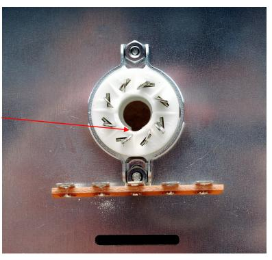
socket mounting screw hole from the top side.
