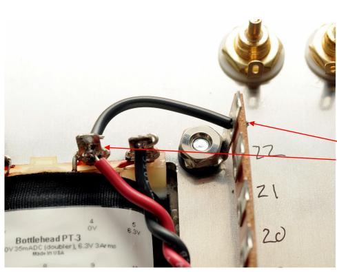
() Cut a 2" (50mm) piece of black wire, strip both ends back 1/4" (6mm). Attach and solder one end to power transformer terminal 4. Attach and solder the other end to terminal 22L.
