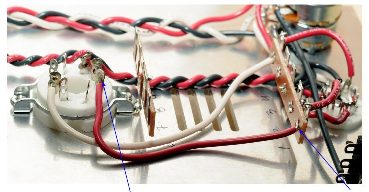
() Cut a 4" (100mm) piece of red wire. Strip both ends 1/4" (6mm). Attach and solder one end to 1L Attach and solder the other end to B1.
