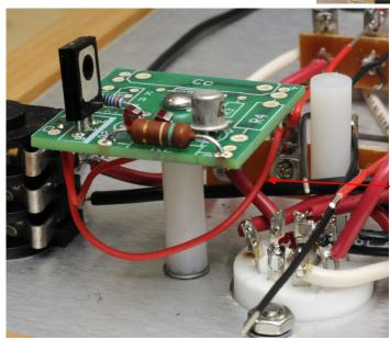
() Attach and solder the inner red wire (from 2U) to the I terminal.
