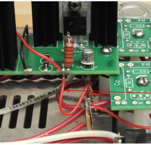
Attach and solder the red wire from 2U to the B+ pad on the left side of the PC board.
