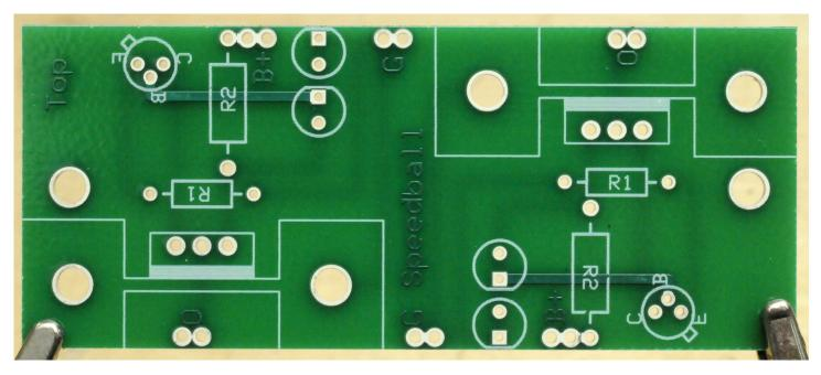
() Install the four HLMP-6000 red LED's with the banded ends in the square solder pads and facing the outside edges of the PC board.
