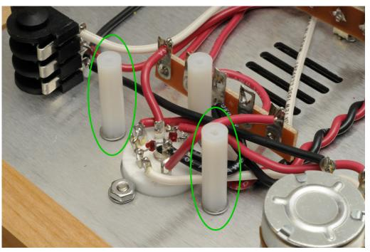
Cut a 2" piece of red wire and strip both ends  $\frac{1}{4}$ ". Attach one end to 2U. Cut a  $\frac{1}{2}$ " piece of black wire and strip both ends  $\frac{1}{4}$ ". Attach and solder one end to 7L.
