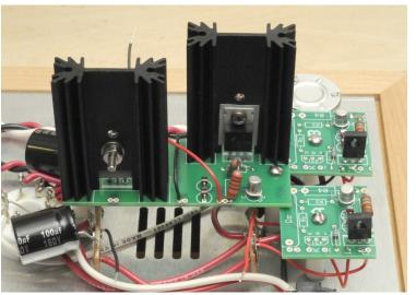
Mount the large PC board with two #4 x  $\frac{1}{4}$ " screws.
