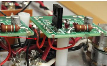
Attach and solder the inner red wire (4U) to the pad labeled I.-
