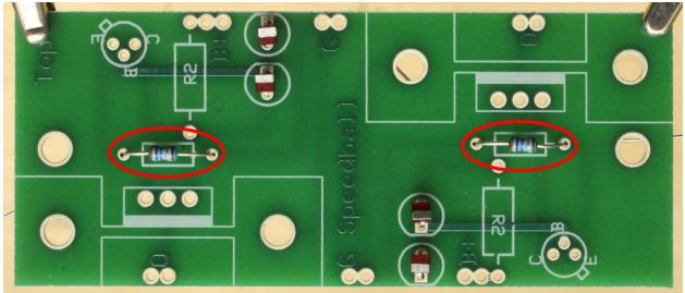
() Install the 31.6 ohm resistors in the R1 positions as shown.
