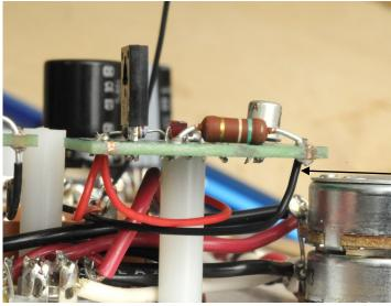
Attach and solder the remaining black wire to the pad labeled G. Note: the "G" may not be visible on the board. The pad is next to the outboard end of the 150K ohm resistor.
