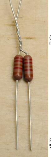
() Twist the leads of two 22.1k <sup>3</sup>/<sub>4</sub> watt resistors together.
