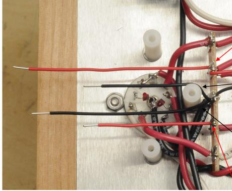
Cut a 3" piece of red wire and strip both ends ¼". Attach one end to 2U and solder 2U.
