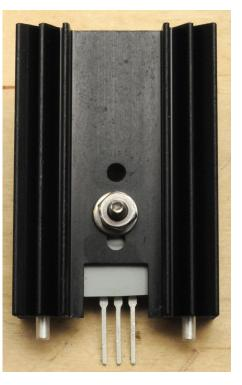
() Secure this assembly snugly with the flat washer, lock washer, and nut in that order.
