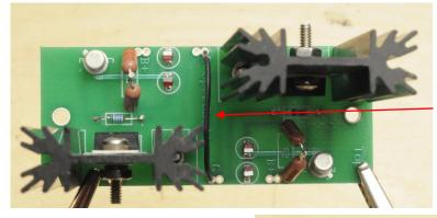
() Cut a 1<sup>3</sup>/<sub>4</sub> " piece of black wire. Strip both ends back <sup>1</sup>/<sub>4</sub>". Jumper between the two center holes that are labeled G on the top side and solder.
