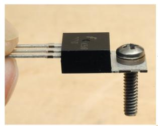
() Upack one transistor mounting kit. Slip the fibre washer onto the bolt provided, then slide the bold through one TIP-50 transistor.
