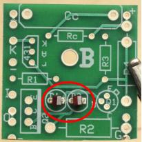
() Install an HLMP-6000 LED in the positions labeled D1 and D2 with the banded end toward the straight edge of the each LED pad.
