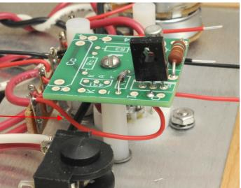
Attach and solder the outermost left red wire (from 1U) to one of the two pads labeled O.-
