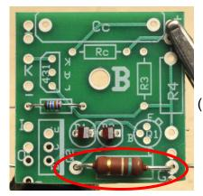
() Install a 150k resistor in the R2 position.
