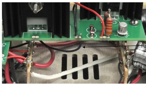
Attach and solder the black wire from 3U to the G pad on the right side of the PC board.
