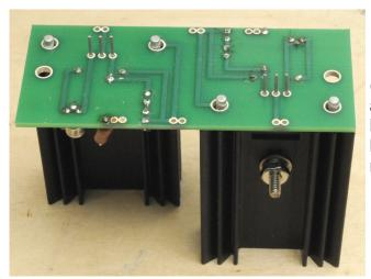
() Install both heatsink/transistor assembliesThis is easiest if you slip the heasink/transistor assemblies onto the board from the top, then flip it over and rest it on the heatsinks themselves.
