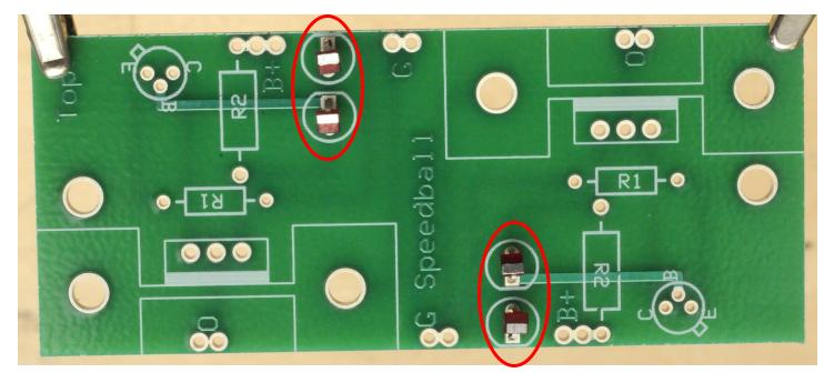
Bending the leads of the various components parallel to the back fo the PC board after insertion will help them stay in place.
