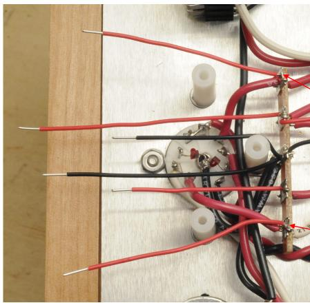
Cut a  $2\frac{1}{4}$  " piece of red wire and strip both ends  $\frac{1}{4}$ ". Attach and solder one end to 1U.
