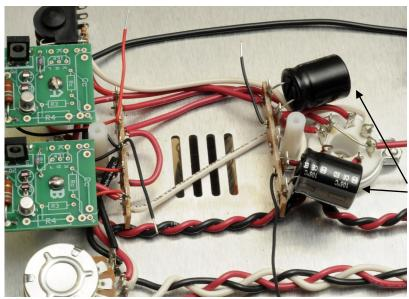
() Bend the remaining four leads toward the edges of the chassis as shown below. Also bend the two 100uf 160v electrolytic capacitors over towards the octal socket.
