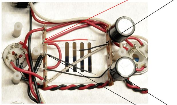
Cut a 3" piece of black wire and strip both ends  $\frac{1}{4}$ ". Attach and solder one end to 9L. Cut a 2" piece of black wire and strip both ends  $\frac{1}{4}$ ". Attach one end to 3U.
