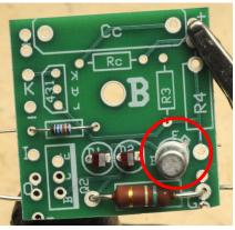
() Install an MJE350 in the Q2 position as shown, with the metalic face of the transistor facing the center of the PC board.
