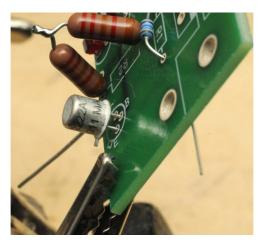
Leave some space between the metal body of the transistor and the PC board
