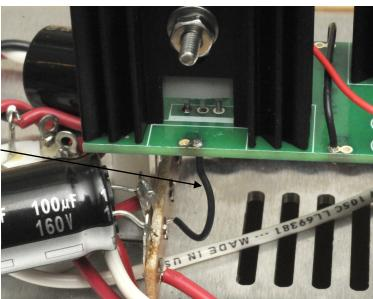
Attach and solder the black wire from 7L to the O pad on the left side of the PC board.
