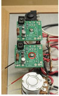
Attach and solder the outermost left red wire (5U) to one of the two pads labeled O.
