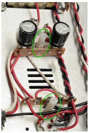
() Install two nylon standoffs, one on the top screw of the 9 pin socket, and one on the bottom screw of the octal socket. Do not remove the nuts before you do this.
