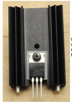
() then mount this assembly through the middle hole in the heatsink.
