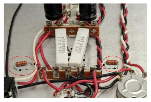
Remove the 3k cathode resistors.
