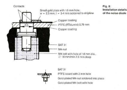
stripline. The small gold plate can be obtained from a connection strip of a power transistor. The dummy is now removed, and the hole is widened from the rear side through the M4-nut with the aid of a 2.1 mm drill, so that one can guarantee that the diode is coupled to the stripline with the aid of the lower cathode connection via the gold plate. With a careful construction, one will achieve a good striplinecoaxial transition.
