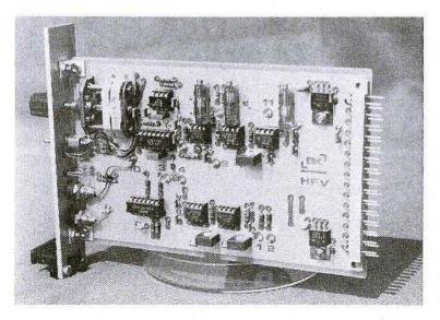
Fig. 33: Photograph of the author's prototype logarithmic module
