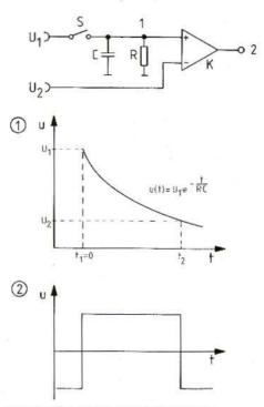
Fig. 31: Principle of the logarithmic circuit
