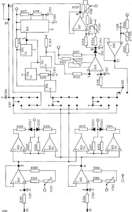
Fig. 32: The logarithmic circuit
