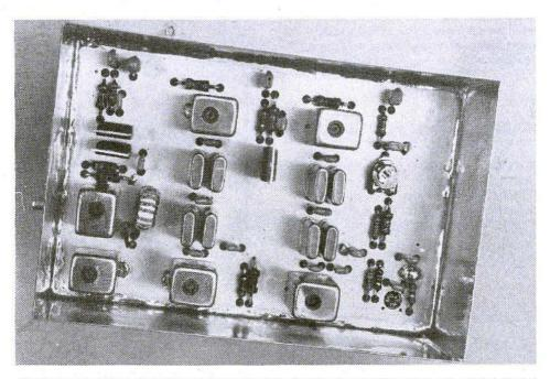
Fig. 1: Photograph of the author's prototype CCW-crystal filter for use as a module in the IF-circuit designed by DJ 3 RV (VHF COMMUNICATIONS 14, Ed. 4/82, Pages 239–252)
