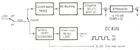
Fig. 4: Block diagram of the noise source and its power supply with switching amplifier
