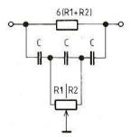
Fig. 9: The (Notch) filter of the VSWR-indicator
