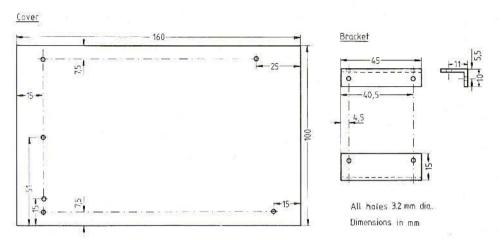
Fig. 27: Mechanical parts for constructing the power supply module
