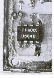
Fig. 4: When correctly installed for UHF, many U 664 B operate up to 1300 MHz
