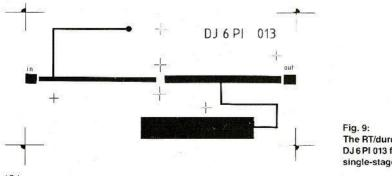
Fig. 9: The RT/duroid PC-board DJ 6 PI 013 for the single-stage FET preamplifier
