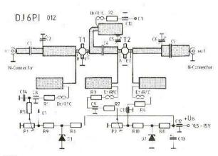
Fig. 1: Two-stage preamplifier for 1.7 GHz equipped with bipolar transistors. NF = 2.4 dB and G = 23 dB
