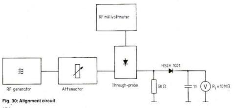
Set the RF-millivoltmeter to its 3 V range and connect a meter to testpoint A of the AF-module. Align P 103 to obtain a voltage of 1 V at this testpoint (full scale).
