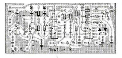
Fig. 3: PC-board and component location plan for the VSWRindicator
