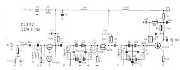
Fig. 4: Circuit diagram of the whole CCW-filter module
