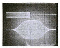
Fig. 5a: Pulse behaviour of the CCW-filter module with input and output pulse displayed linearly. Pulse duration: 12.5 ms; time scale: 2.5 ms/division
