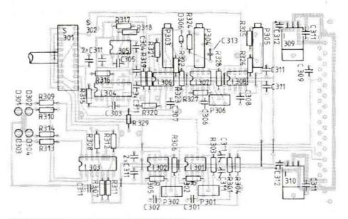
Fig. 34: Components on the logarithmic board DL 0 HV 003
