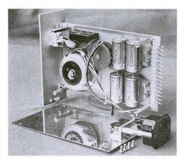
Fig. 26: Photograph of the open power supply module
