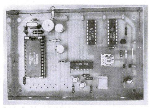
Fig. 5: One will see the input circuit of the U 664 B of the counter module
