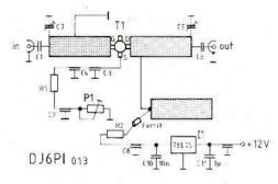
the transistor itself, that determines the noise figure, but also the microwave trimmer used at the input, the disk capacitors and their construction, the quality of the connectors, as well as finally the actual alignment. For this reason, the following sections are very important.
