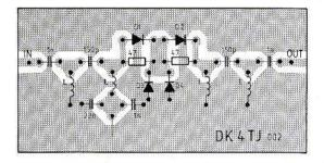
Fig. 6: PC-board and component location plan for the modulator shown in Figure 4
