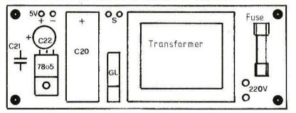
Fig. 7: Power supply board DCØRZ 004 is able to provide 300 mA at +5 V
