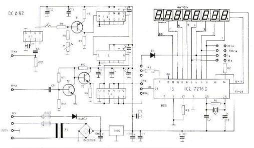
Fig. 2: Circuit diagram of the counter with eight-digit readout and power supply
