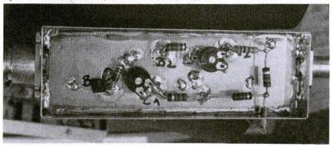
Fig. 7: The DC-voltage network can be accommodated on the ground side of the board between the feedthrough capacitors and the ground surface
