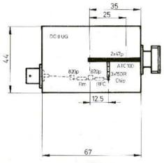
Fig. 7: Layout of a 0.79 mm RT/duroid board 140
