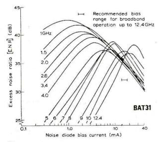
Fig. 3: Noise power as a function of avalanche current with frequ
