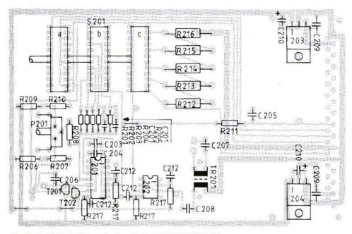
Fig. 18: Components of the control module (mechanical) DL 0 HV 002
