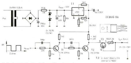
Fig. 6: Power supply with switching amplifier and current source
