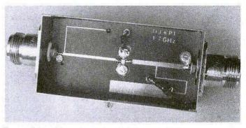
Fig. 11: A few, high-quality components are required for the 1 dB preamplifier
