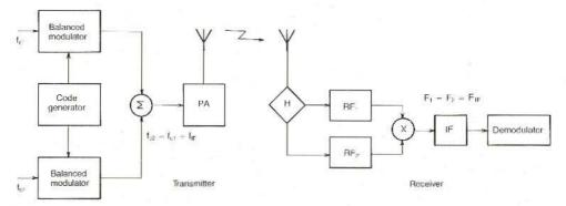
Fig. 11: Synchronization method using a transmitted reference signal
