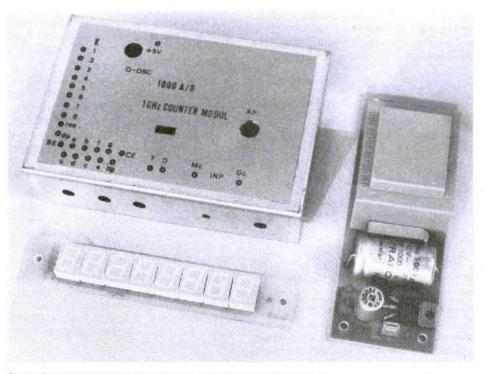
Fig. 1: Counter module, readout, and power supply before the connection
