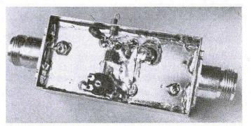
Fig. 12: The DC-voltage network is accommodated in the 10 mm high ground-side of the case
