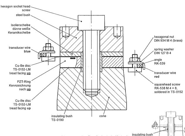
RK 100 SH from serial no. 192 178 xxx (onwards): an epoxy glass fibre disc is attached instead of the white ring IS 013. If the oscillating system is damaged, the entire set of replacements parts must be used. If necessary re-adjust the generator.
