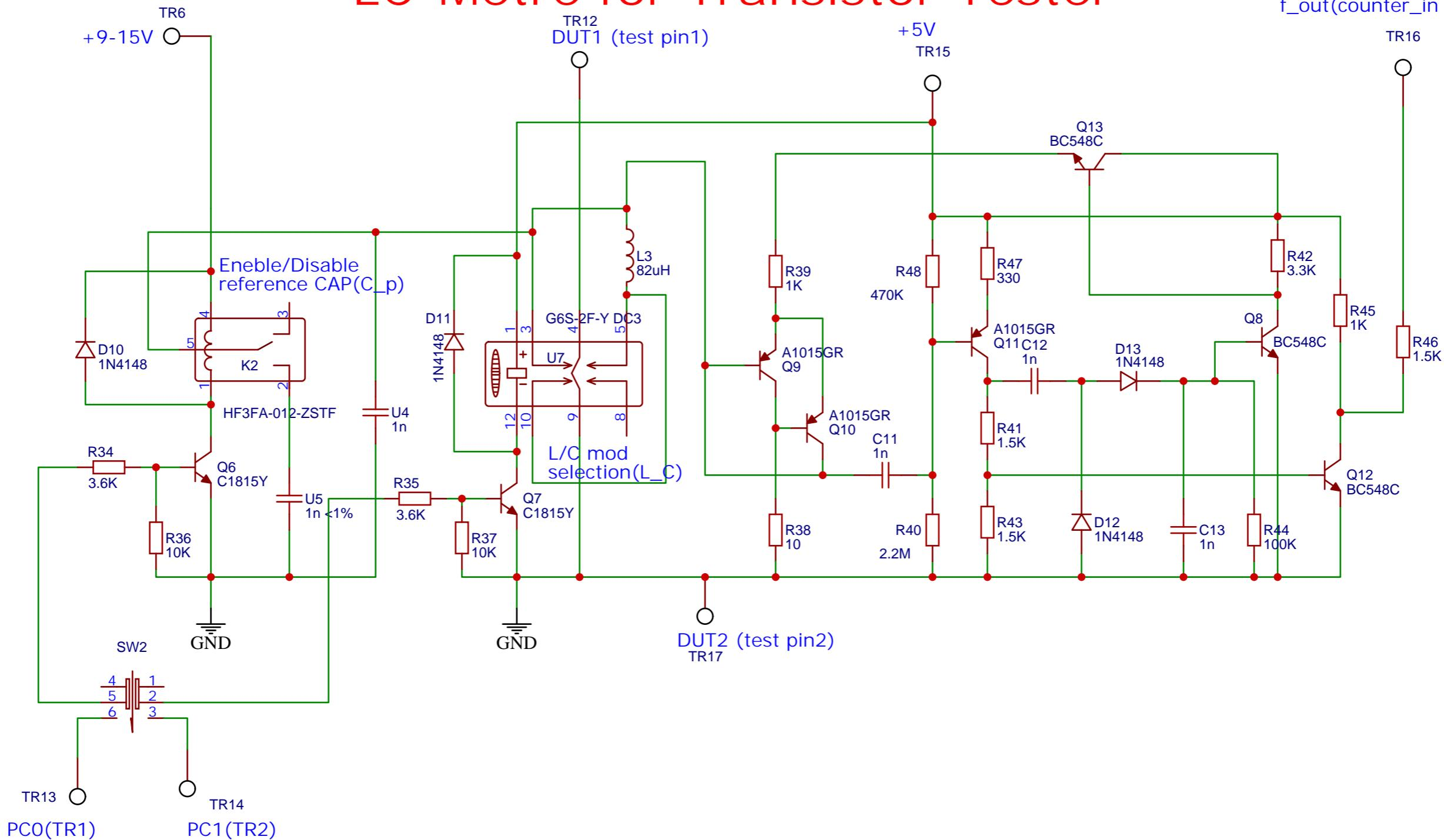
For correct operation of the device, the input of the frequency meter PD4 must not be connected to the display.
