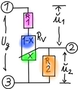
$$\frac{\check{u}_1(1-2)}{\check{u}_2(2-3)} = \left( \frac{(R_1 + (1-x) \cdot R_v)}{\left( \frac{x \cdot R_v \cdot R_2}{(x \cdot R_v + R_2)} \right)} \right)$$
