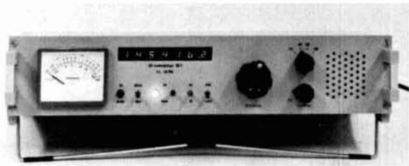
fig. 2. Photograph of a semi-synthesized 2-meter transceiver using the converter shown in fig. 1.
