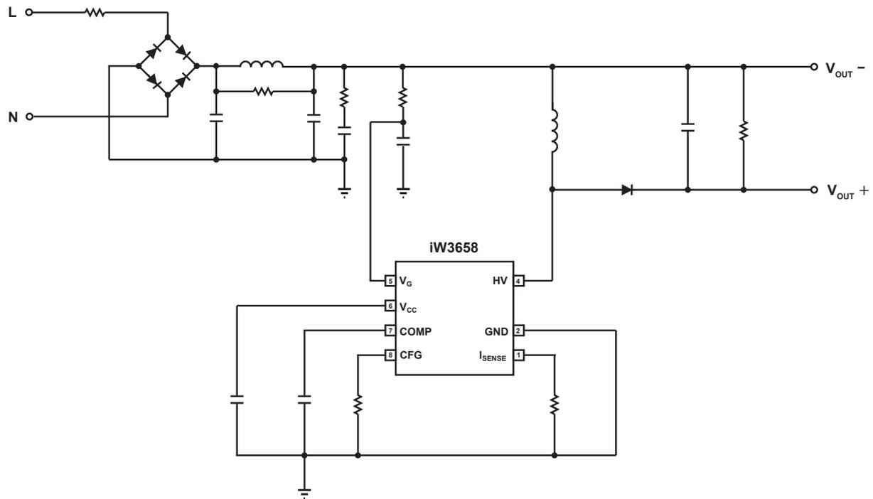
Figure 3.1 : iW3658 Typical Application Circuit
