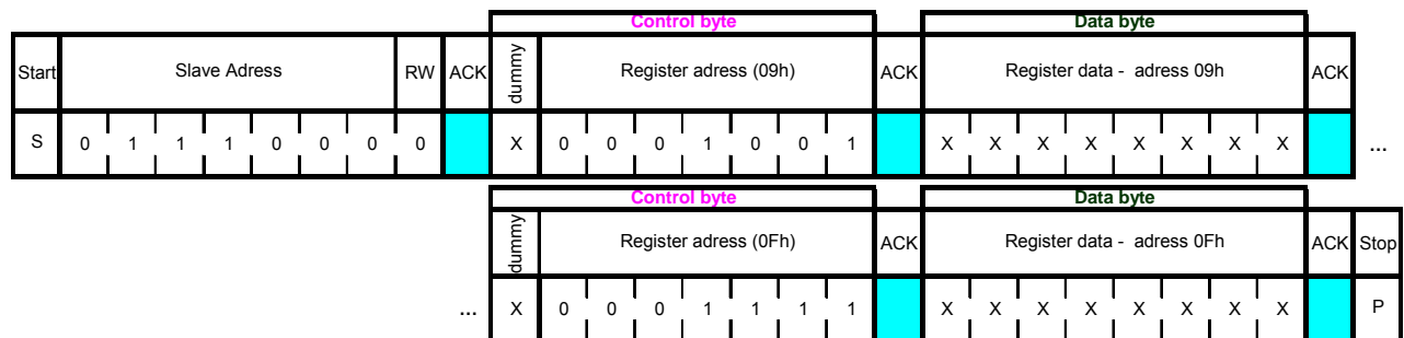
Figure 15: I 2 C multiple write protocol
