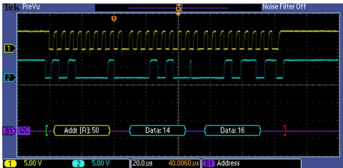
Triggering on a specific data packet going across an I2C bus. The yellow waveform is clock and the blue waveform is data. A bus waveform provides decoded packet content including Start, Address, Read/Write, Data, and Stop.
