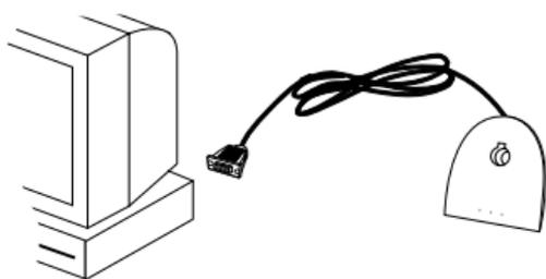
1. Insert the Cyberwell cable into the the COM1 port on the back of your PC. If the COM1 port is in use, use the COM2 port.
