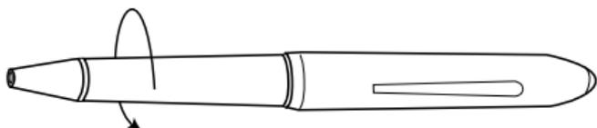
2. Insert the batteries one at a time with the positive (+) end up into the clip end of the pen:
