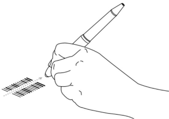
A successful read of the bar code is indicated by an audible beep and a green LED. If you do not hear a beep, try scanning again, using a different speed, or following a different path through the bar code.
