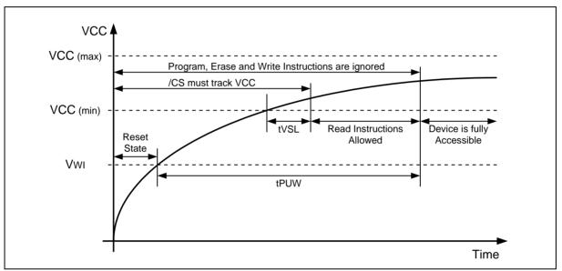
Figure 58. Power-up Timing and Voltage Levels
