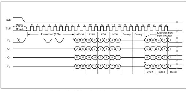
Figure 24a. Fast Read Quad I/O Instruction (Initial instruction or previous M5-4≠10) 32-Bit Address is required when the device is operating in 4-Byte Address Mode
