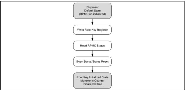
Figure 3a. W25R256JW RPMC Initialization Flow Diagram
