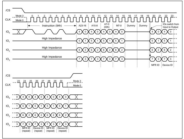
Figure 41. Read Manufacturer / Device ID Quad I/O Instruction 32-Bit Address is required when the device is operating in 4-Byte Address Mode
