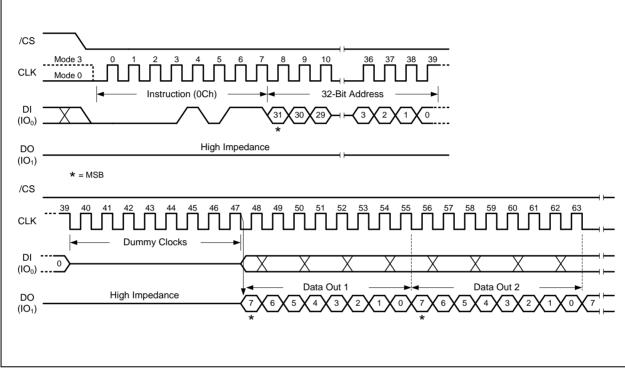
Figure 17. Fast Read with 4-Byte Address Instruction
