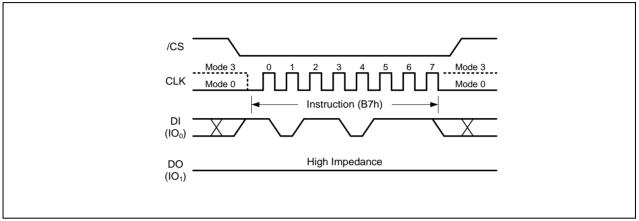
Figure 12. Enter 4-Byte Address Mode instruction
