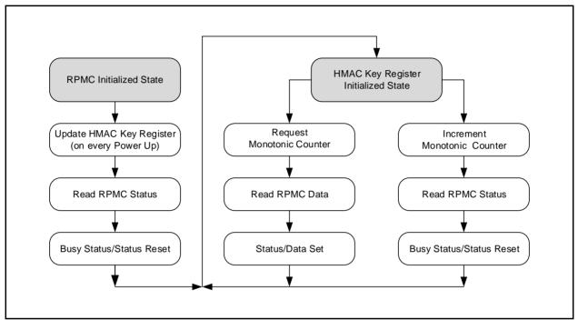
Figure 3b. W25R256JW RPMC Operation Flow Diagram
