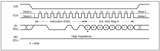
Figure 11a. Write Extended Address Register Instruction
