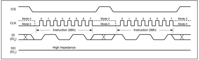
Figure 57a. Enable Reset and Reset Instruction Sequence
