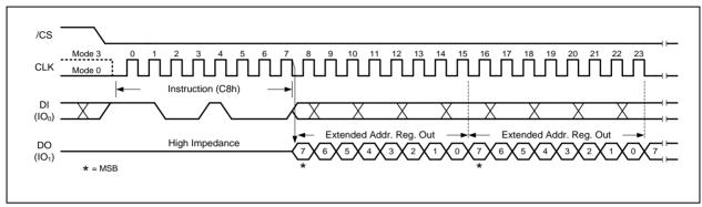
Figure 10a. Read Extended Address Register Instruction
