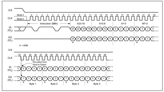
Figure 22a. Fast Read Dual I/O Instruction (Initial instruction or previous M5-4  $\neq$  10) 32-Bit Address is required when the device is operating in 4-Byte Address Mode
