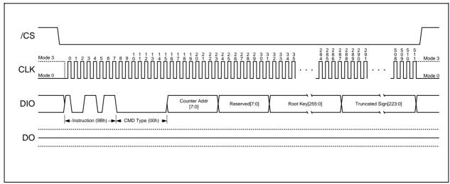
Figure 43. Write Root Key Register Instruction
