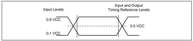
Figure 59. AC Measurement I/O Waveform
