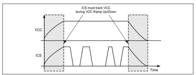
Figure 58b. Power-up, Power-Down Requirement
