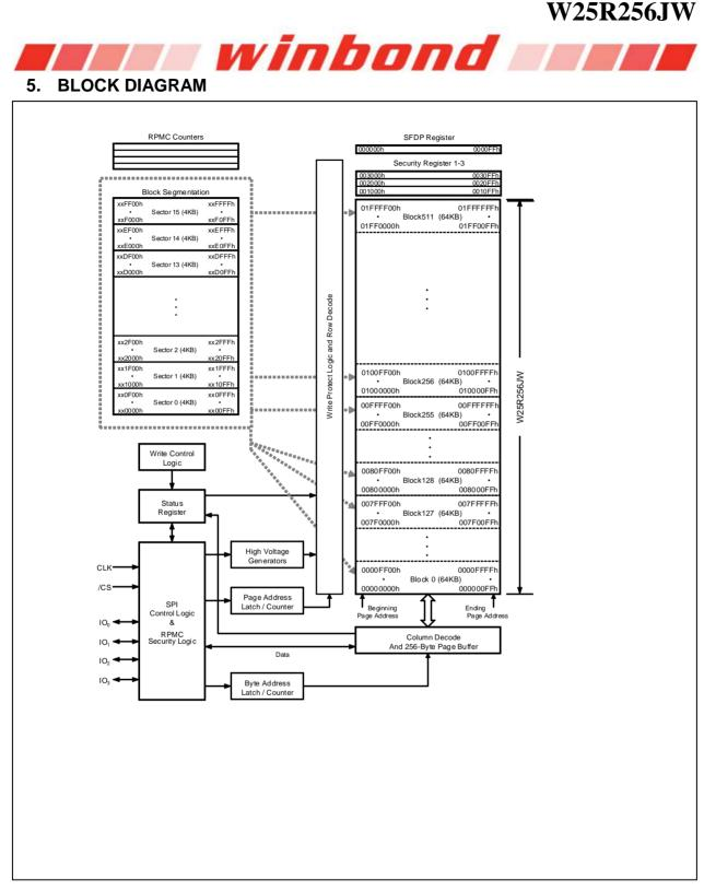
Figure 2. W25R256JW Serial Flash Memory Block Diagram
