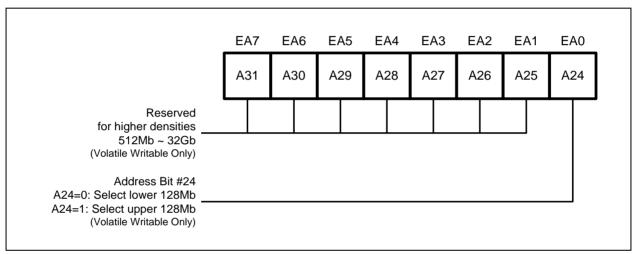
Figure 4e. Extended Address Register
