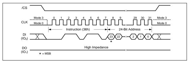
Figure 52a. Individual Block/Sector Lock Instruction 32-Bit Address is required when the device is operating in 4-Byte Address Mode
