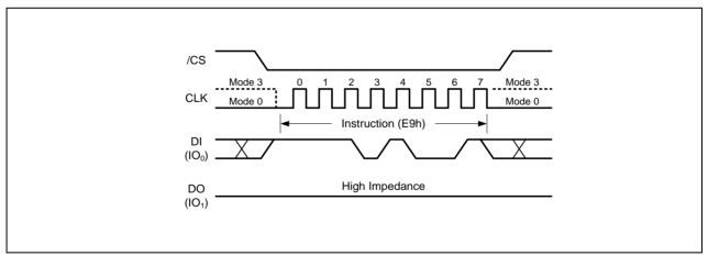
Figure 13. Exit 4-Byte Address Mode instruction
