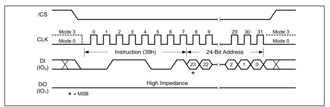
Figure 53a. Individual Block Unlock Instruction 32-Bit Address is required when the device is operating in 4-Byte Address Mode **\_\_\_\_** winbond **\_\_**
