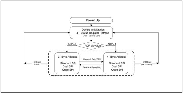
Figure 3. W25R256JW Serial Flash Memory Operation Diagram
