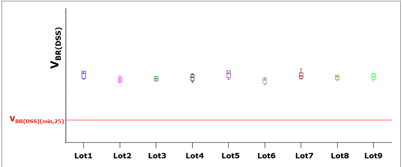
Figure 8 Example of production distribution for V_{BR(DSS)}
