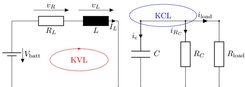
**Figure 5.6** – Equivalent circuit of the step-up DC-DC converter: T1 OFF and T2 ON.
