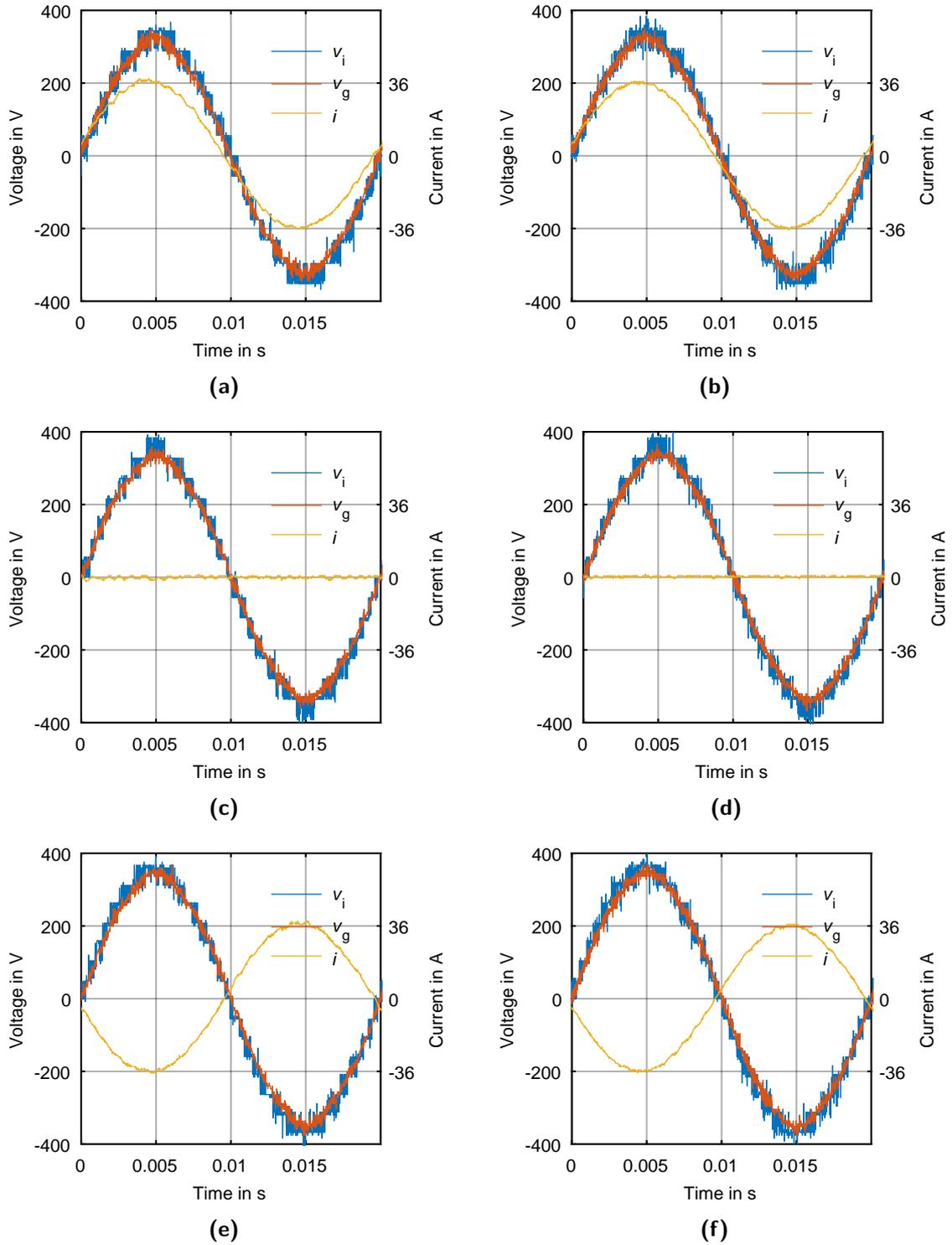
**Figure 7.26** – Inverter  $v_i$  and grid  $v_g$  voltages and current  $i$  measurement results using the CHB inverter prototype at  $f_{sw} = 16$  kHz (a) while charging, (c) at zero current, (e) while discharging, at  $f_{sw} = 32$  kHz (b) while charging, (d) at zero current, and (f) while discharging at constant filter value of 0.98 mH.
