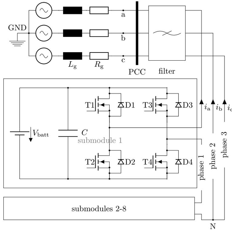
**Figure 5.1** – Circuit of the one-stage CHB inverter topology [100].
