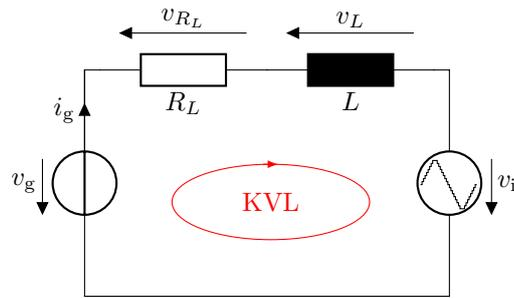
**Figure 7.17** – Single phase equivalent circuit of the CHB inverter connected to the grid through L-filter.
