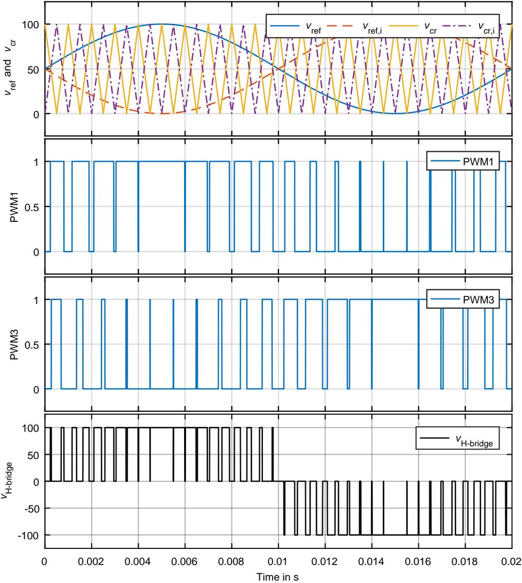
**Figure 3.3** – H-bridge inverter unipolar PWM function principle using ideal sinusoidal signal with fundamental frequency  $f_{ref} = 50\text{ Hz}$  and carrier-signal with switching frequency of  $f_{sw} = 1\text{ kHz}$  (top plot). Both plots in the middle represent pulse signals for switches S1 and S3. The bottom plot shows the resulting three-level H-bridge inverter output voltage using unipolar PWM [16] [126] [181].
