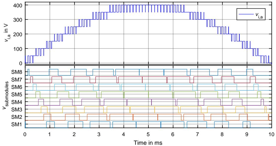
**Figure 7.6** – CHB inverter and submodules voltages using PSPWM.
