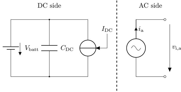
**Figure 8.1** – Average model of a single-phase DC-AC inverter, e.g. H-bridge inverter.
