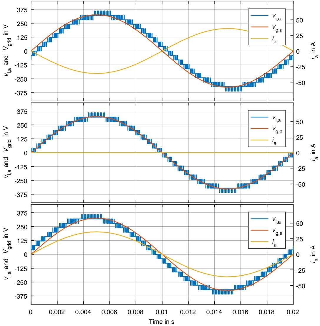
**Figure 5.16** – Two-stage CHB inverter and grid voltages and current using step-down DC-DC converter. The CHB inverter requires 17 voltage levels while charging and discharging the battery modules and when the phase current is set to zero.
