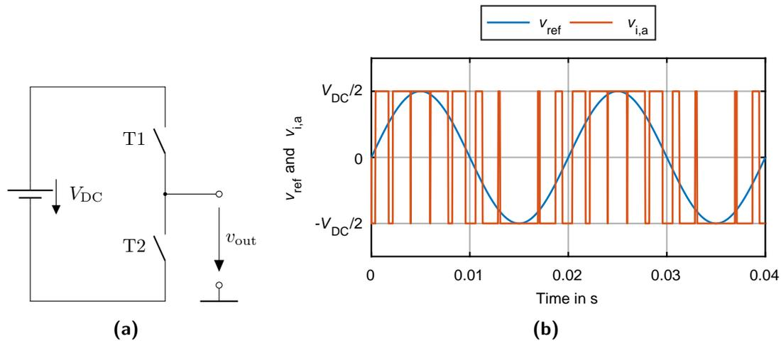
Figure 4.1 – Schematic circuit for two-level inverter and its output voltages [183].
