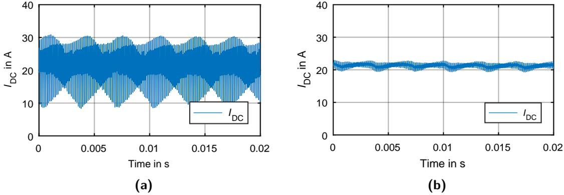
**Figure 3.11** – B6-bridge inverter DC-link current using different capacitance values of (a) 0.14 mF (b) and 1.4 mF.
