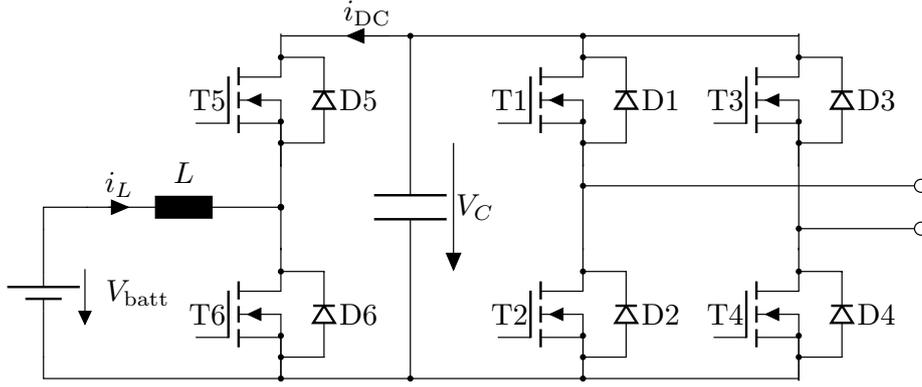
**Figure 5.3** – Circuit of the two-stage CHB inverter's submodule including the bidirectional step-up DC-DC converter.
