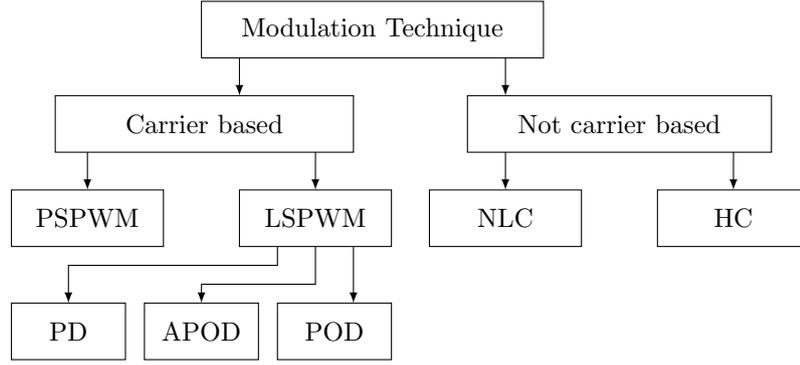
**Figure 7.4** – Modulation techniques for the CHB inverter on circuit-level.
