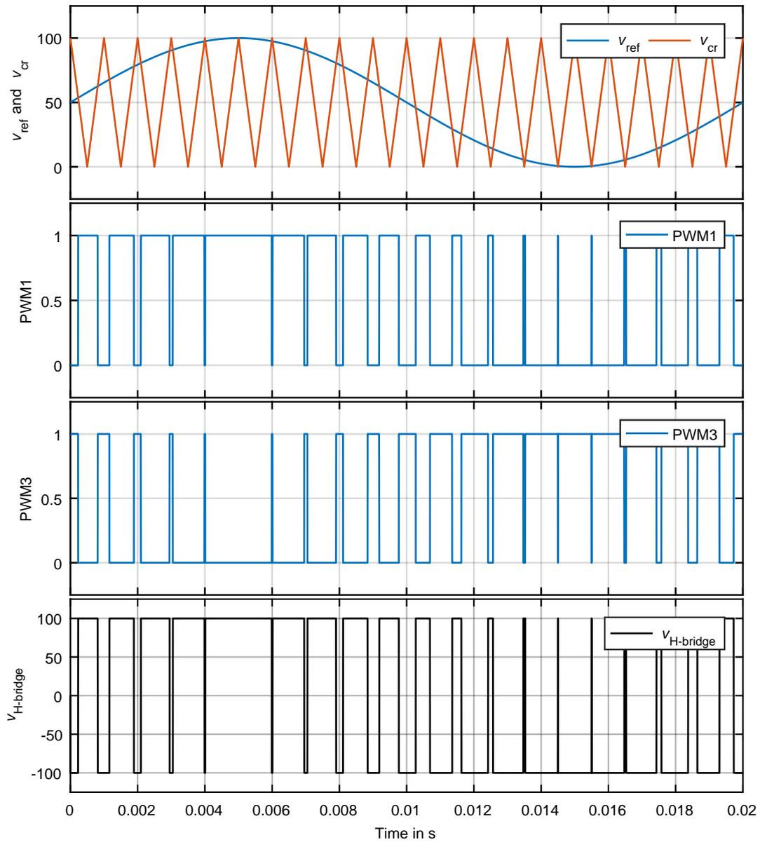
**Figure 3.2** – H-bridge inverter bipolar PWM function principle using ideal sinusoidal signal with fundamental frequency  $f_{ref} = 50$  Hz and carrier-signal with switching frequency of  $f_{sw} = 1$  kHz (top plot). Both plots in the middle represent pulse signals for switches S1 and S3. The bottom plot shows the resulting two-level H-bridge inverter output voltage using bipolar PWM [16] [126] [181].
