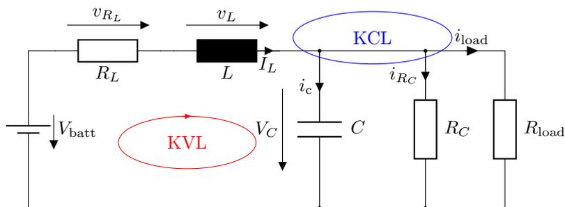
**Figure 5.5** – Equivalent circuit of the step-up DC-DC converter: T1 ON and T2 OFF.
