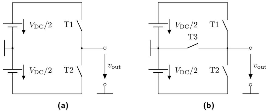
Figure 4.3 – Two- and three-level inverter topologies.
