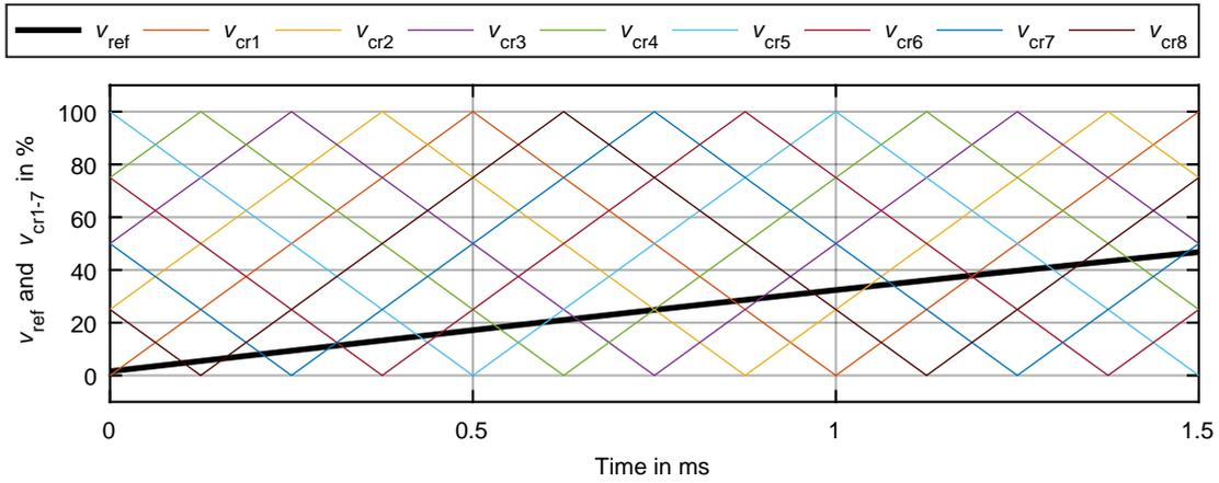
**Figure 7.5** – Reference voltages and carrier-signals for the 17-level CHB inverter using PSPWM.
