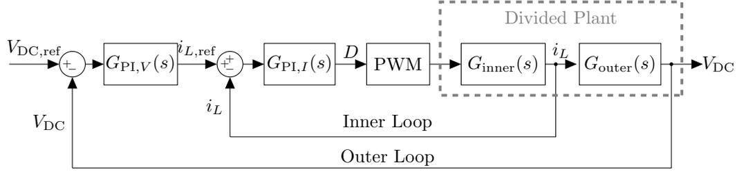
**Figure 5.8** – Detailed cascaded control structure of the step-up DC-DC converter.
