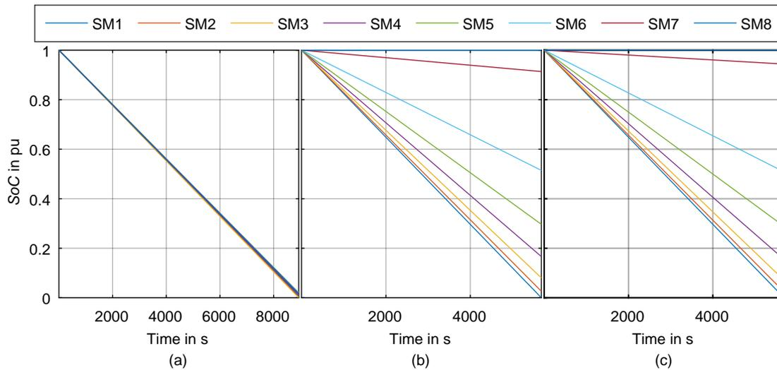
**Figure 8.7** – State of charge of the battery modules of phase a using simulation on circuit-level using: (a) PSPWM, (b) PD-LSPWM, and (c) NLC.
