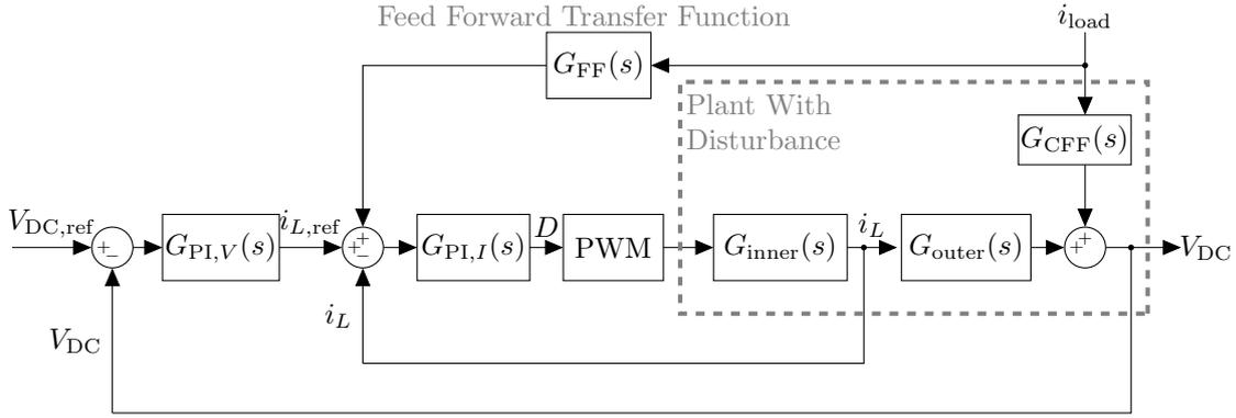
**Figure 5.12** – Detailed cascaded control structure using feed forward control and considering the plant with disturbance [107].
