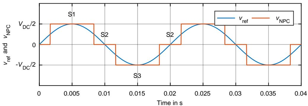
Figure 4.7 – Output voltage of the circuit in Fig. 4.6 with the switching states in Table 4.3.
