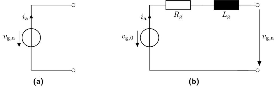
**Figure 7.2** – Single-phase (a) ideal grid model represented by a voltage source, (b) strong, and weak grid models containing internal resistance and inductance.
