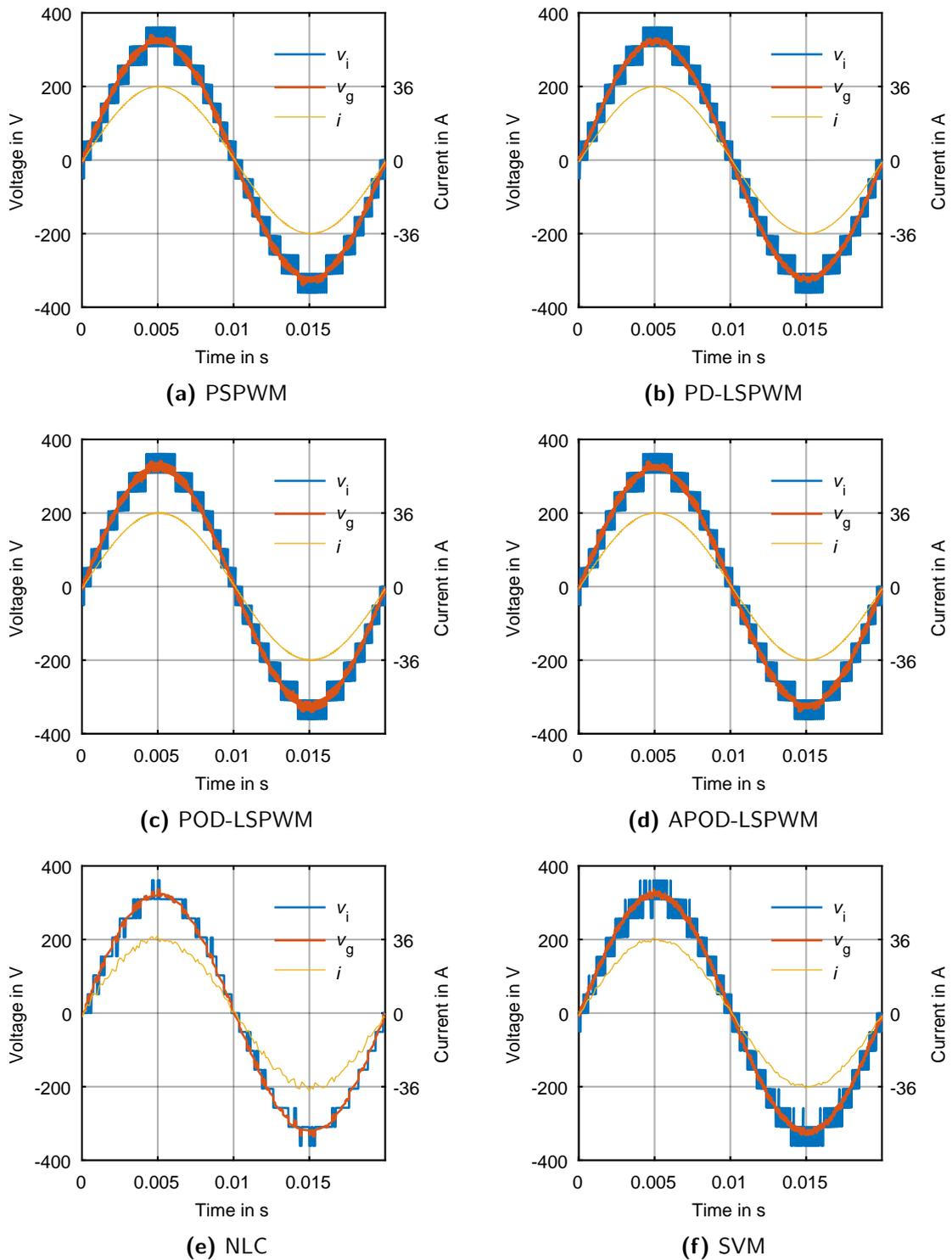
**Figure 7.23** – CHB inverter and grid voltages and phase current using different modulation techniques during the charging operation.
