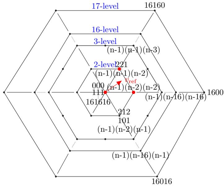
**Figure 7.12** – Space vector diagram of the 17-level CHB inverter.
