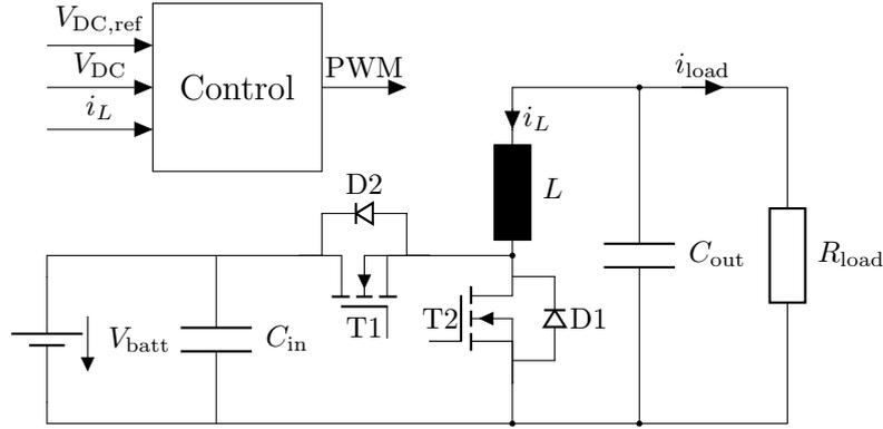
**Figure 5.15** – Circuit of the used bidirectional step-down DC-DC converter between the H-bridge inverter and the battery modules in the CHB inverter.
