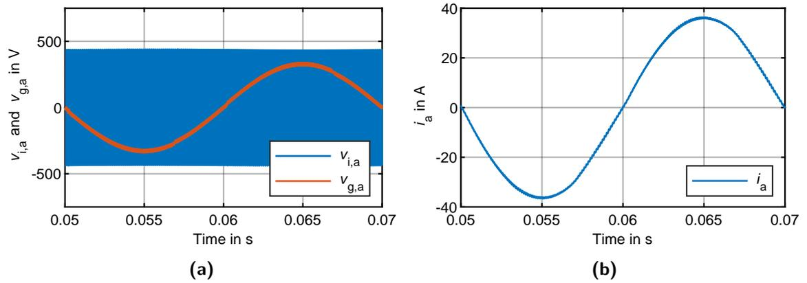
**Figure 3.10** – B6-bridge (a) inverter  $v_{i,a}$  and grid voltages  $v_{g,a}$  (b) and AC current  $i_a$  during the charging operation of the BESS.
