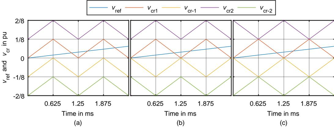
**Figure 7.7** – Reference voltages and carrier-signals for the 17-level CHB inverter using (a) PD-, (b) POD-, and (c) APOD-LSPWM.
