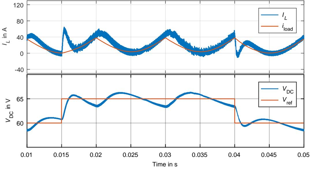
**Figure 5.11** – Step-up DC-DC converter's inductor current  $I_L$  and DC-link voltage  $V_{DC}$  in case of non-linear load without feed-forward control [107].
