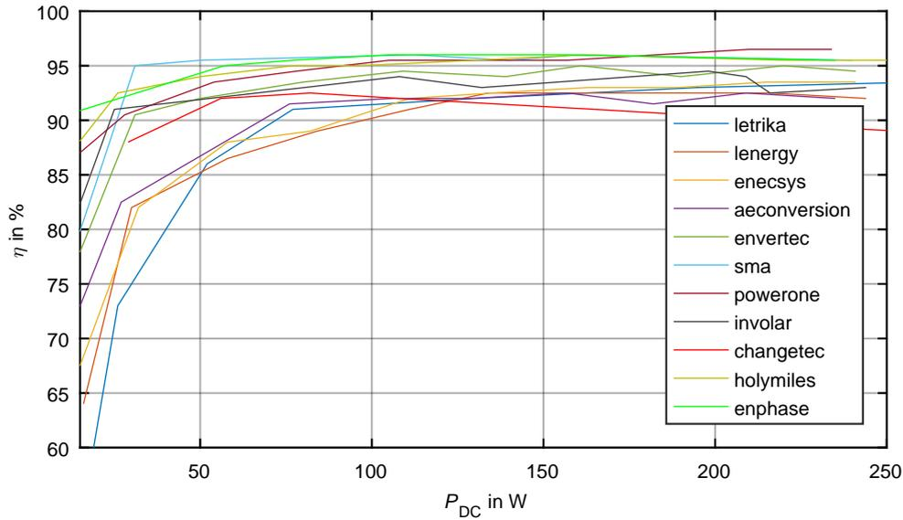
**Figure 3.7** – Measured DC-AC conversion efficiencies as a function of DC input power for eleven micro-inverters with single PV module inputs [37].
