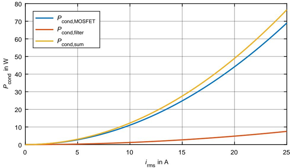
**Figure 6.2** – Conduction power losses for the internal resistance of the power switches and the power filter depending on the current rms value.
