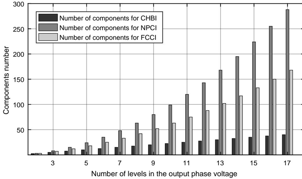
**Figure 4.10** – A comparison between the number of components in different multilevel inverter topologies [20].
