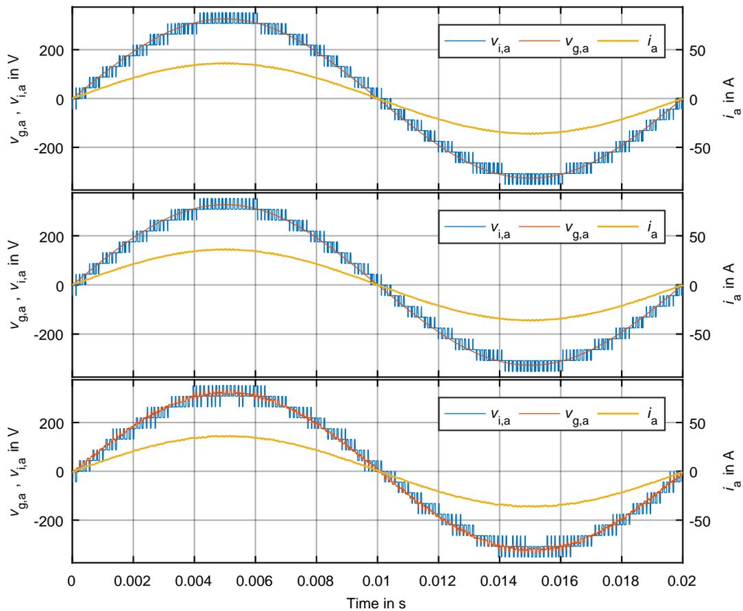
**Figure 7.3** – Grid and inverter voltages and current using ideal, strong, and weak grid model.
