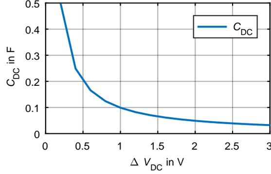
**Figure 3.5** – Sizing the DC-link capacitance to decrease the voltage ripple  $\Delta V_{DC}$  around a nominal voltage of 50 V.
