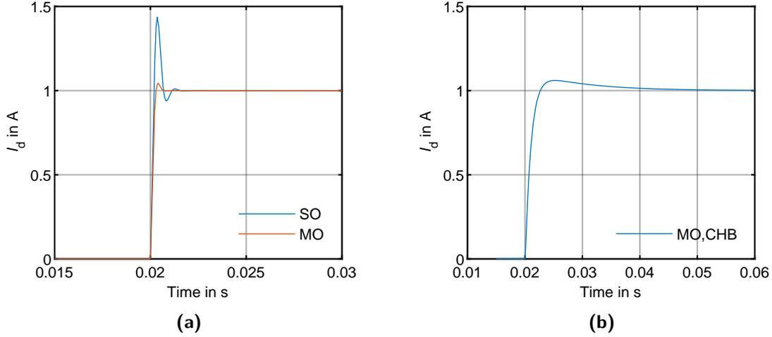
**Figure 7.20** – Step responses of the closed loop using (a) SO, MO, and (b) MOCHB.
