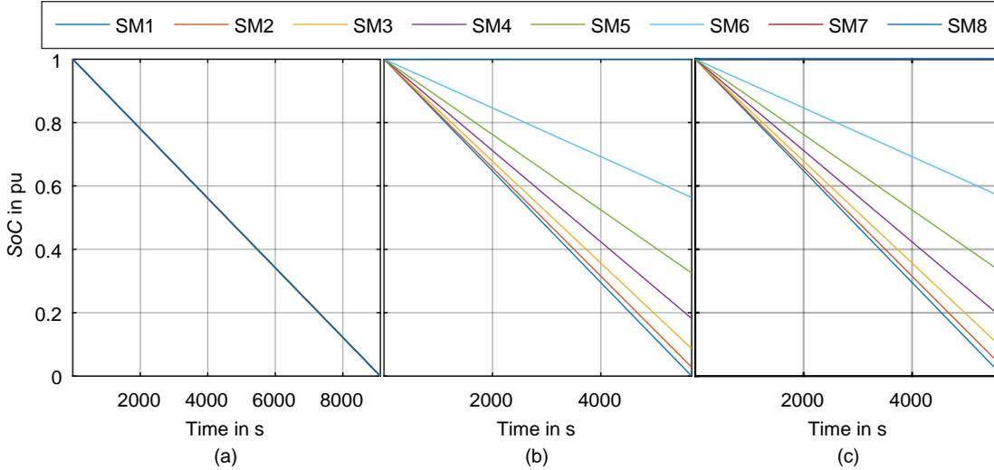
**Figure 8.6** – State of charge of the battery modules of phase a using simulation on system-level using: (a) PSPWM, (b) PD-LSPWM, and (c) NLC.
