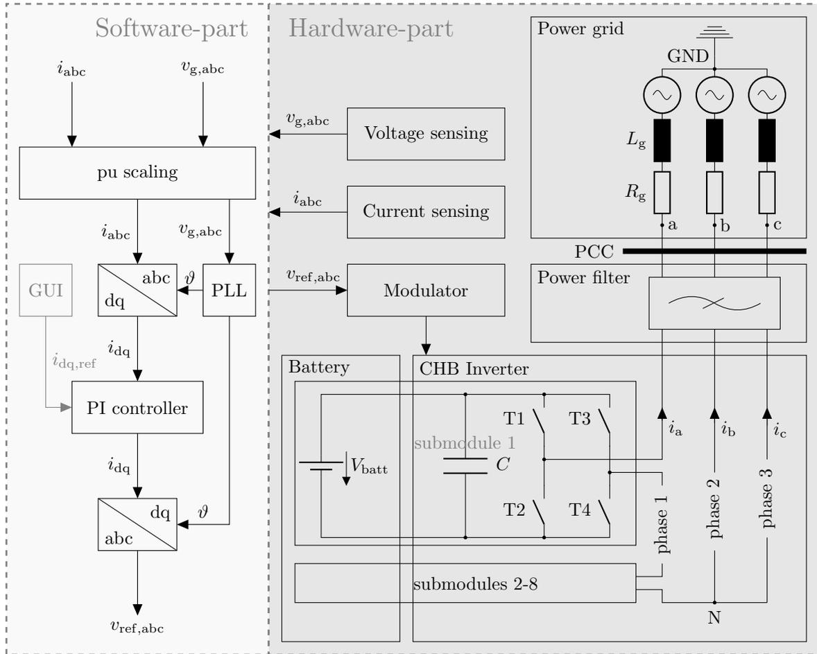
**Figure 7.1** – Simulation model of the CHB inverter on circuit-level.
