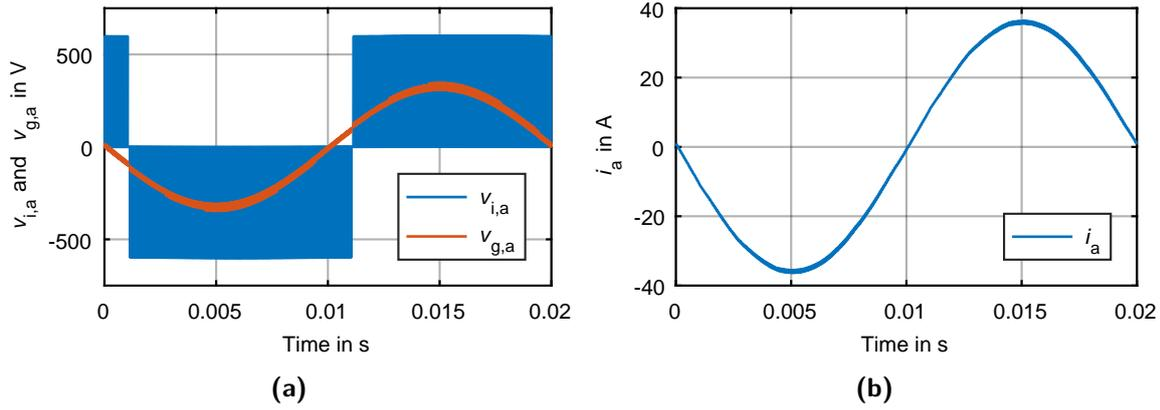
**Figure 3.4** – H-bridge (a) inverter  $v_{i,a}$  and grid voltages  $v_{g,a}$  (b) and AC current  $i_a$  during the charging operation of the BESS.
