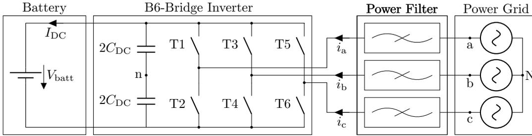
**Figure 3.8** – System overview of conventional three-phase B6-bridge inverter for battery energy storage system.
