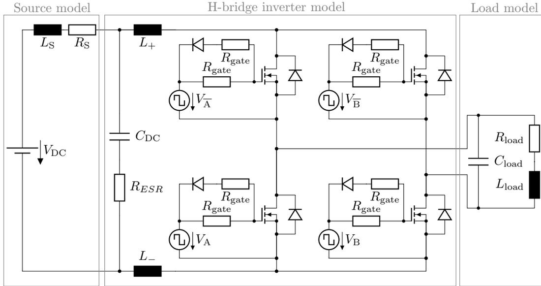
**Figure 6.6** – Circuit used for efficiency simulations on component-level. It considers the PCB parasitic inductances  $L_+$ ,  $L_-$ , the source inductance and resistance  $L_S$ ,  $R_S$ , and the load model represented by a power resistor  $R_{load}$  with its parasitic components  $L_{load}$  and  $C_{load}$  [105].
