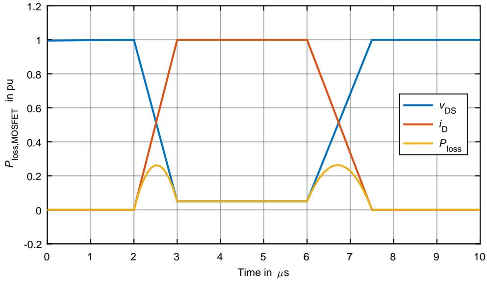
**Figure 6.3** – Idealized power semiconductor dynamic switch-on and -off behaviors [105].
