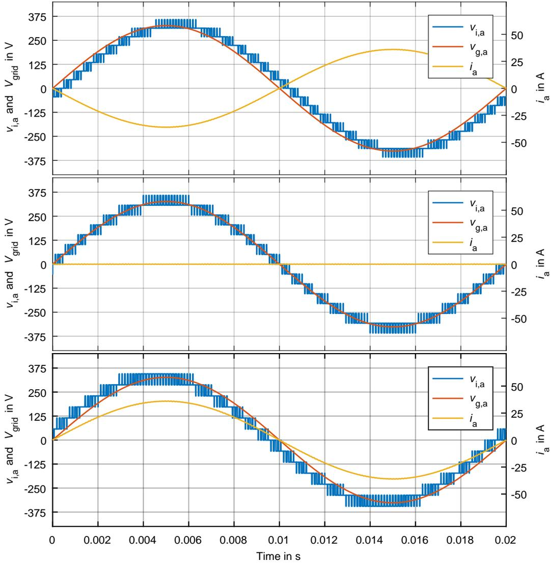
**Figure 5.2** – One-stage CHB inverter and grid voltages and current at different battery voltages. The CHB inverter requires 17 levels at  $V_{batt,min}$  while discharging the BESS (top). It requires 15 levels at  $V_{batt,nom}$  to keep the grid current at zero (middle) and 13 voltage levels at  $V_{batt,max}$  while charging the BESS (bottom). [100].
