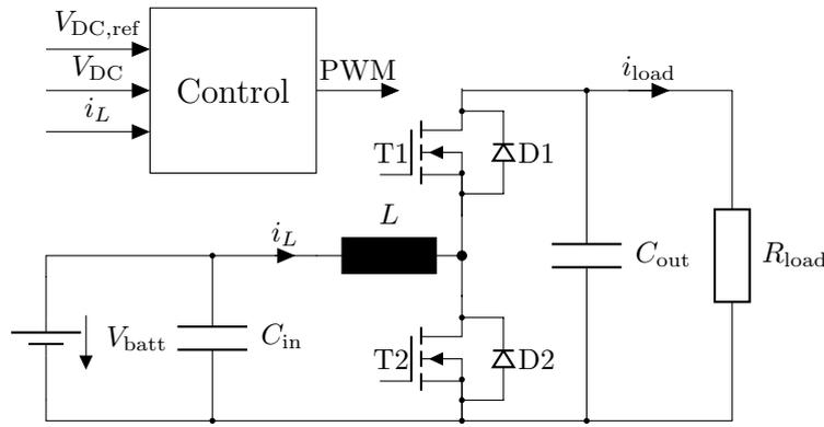
**Figure 5.4** – Circuit of the used bidirectional step-up DC-DC converter between the H-bridge inverter and the battery modules in the CHB inverter.
