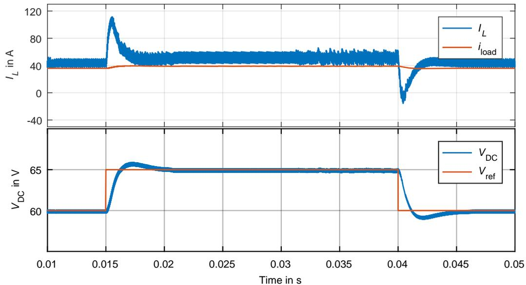
Figure 5.10 – Step-up DC-DC converter's inductor current  $I_L$  and DC-link voltage  $V_{DC}$  in case of linear load without feed-forward control [107].
