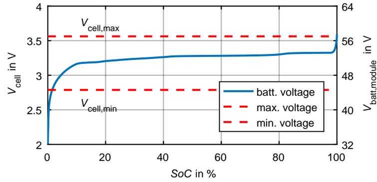
**Figure 3.9** – Measured cell open-circuit voltage and operation range limits.
