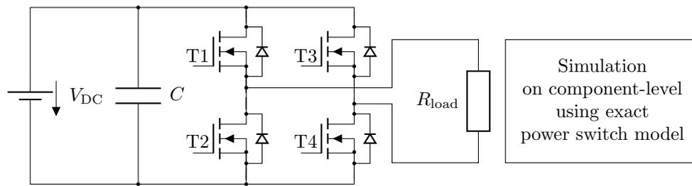
**Figure 6.1** – Simulation on component-level using an exact H-bridge inverter's model [105]
