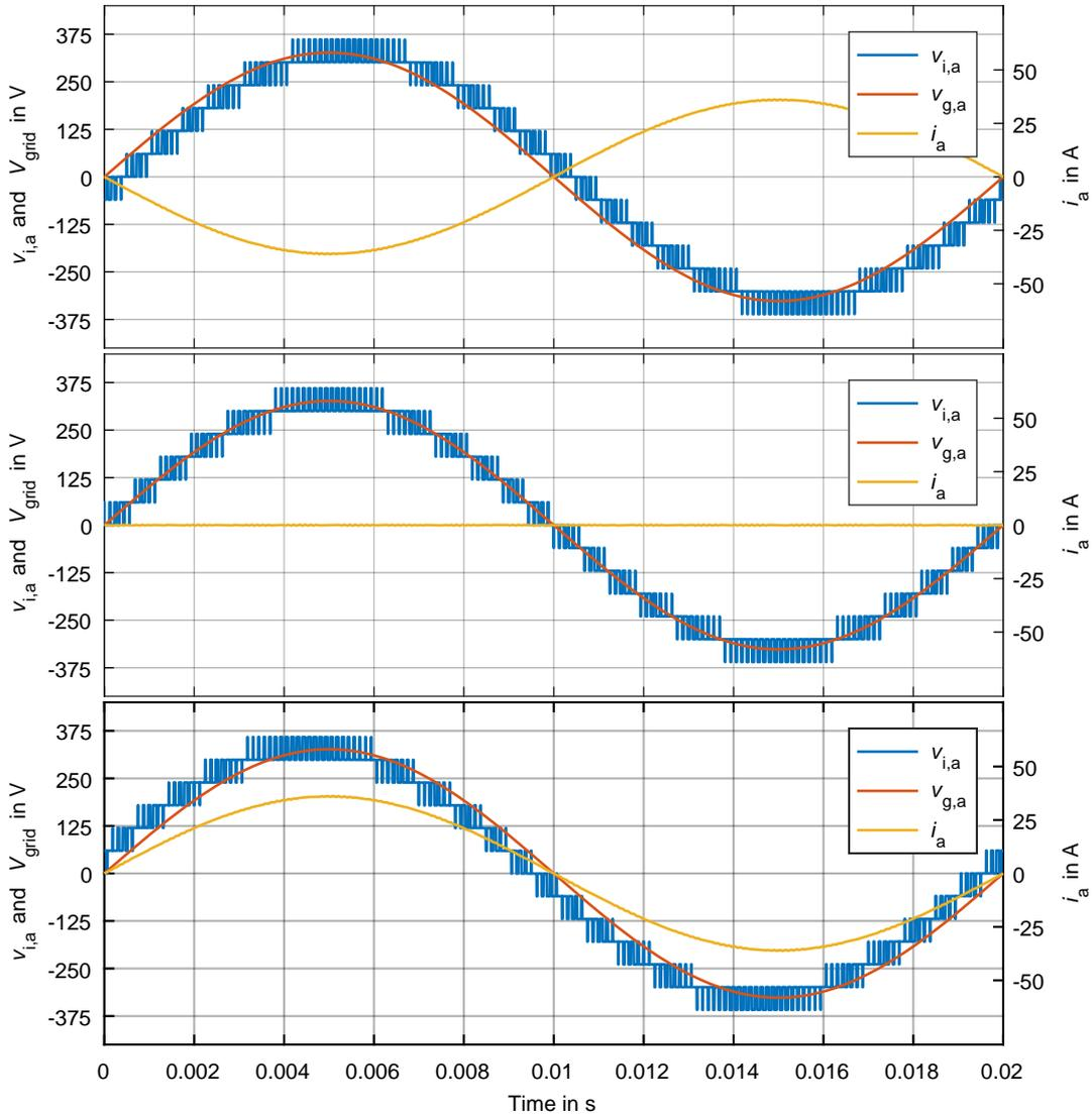
**Figure 5.14** – Two-stage CHB inverter and grid voltages and current using the step-up DC-DC converter. The CHB inverter requires 13 voltage levels while charging and discharging the battery modules and when the phase current is set to zero.
