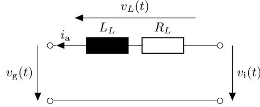
**Figure 7.13** – Equivalent circuit of a power filter.
