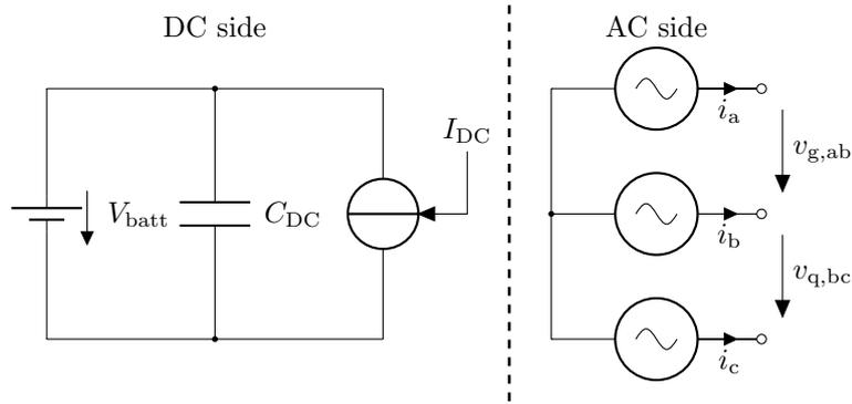
**Figure 8.2** – Average model of a three-phase DC-AC inverter, e.g. B6-bridge inverter.
