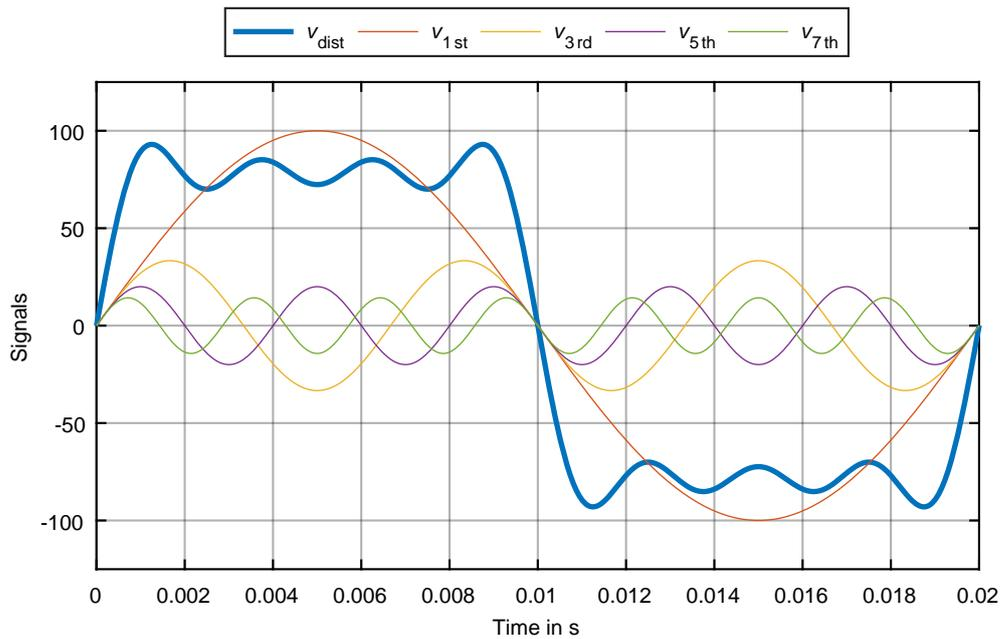
**Figure 2.4** – Addition of the 3<sup>rd</sup>, 5<sup>th</sup>, and 7<sup>th</sup> harmonic to an ideal sine wave and the resulting signal.
