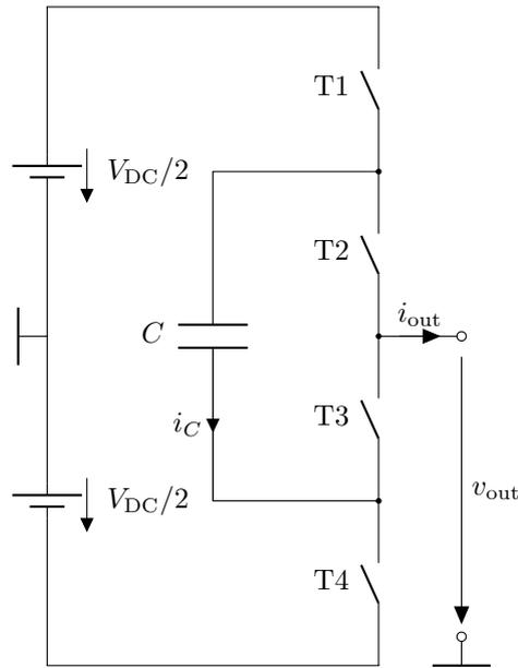
**Figure 4.8** – Basic circuit of three-level flying capacitor clamped inverter.
