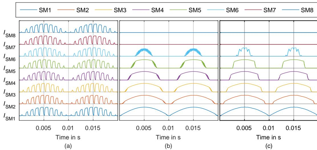
**Figure 8.5** – DC-link current of the submodules of phase a using simulation on circuit-level using: (a) PSPWM, (b) PD-LSPWM, and (c) NLC.
