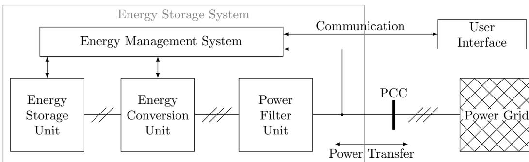
**Figure 2.1** – Schematic diagram of the main components of grid connected energy storage systems.
