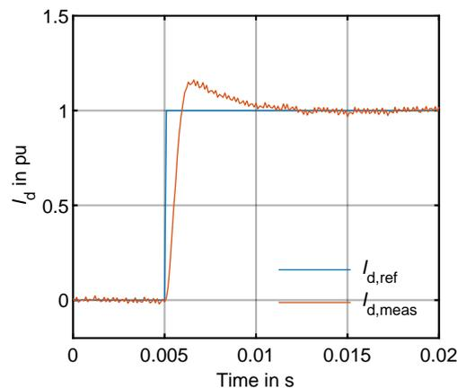
Figure 7.25 – CHB inverter's step response in the hardware.
