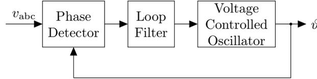
**Figure 7.15** – Structure of non-linear closed control loop in PLL.
