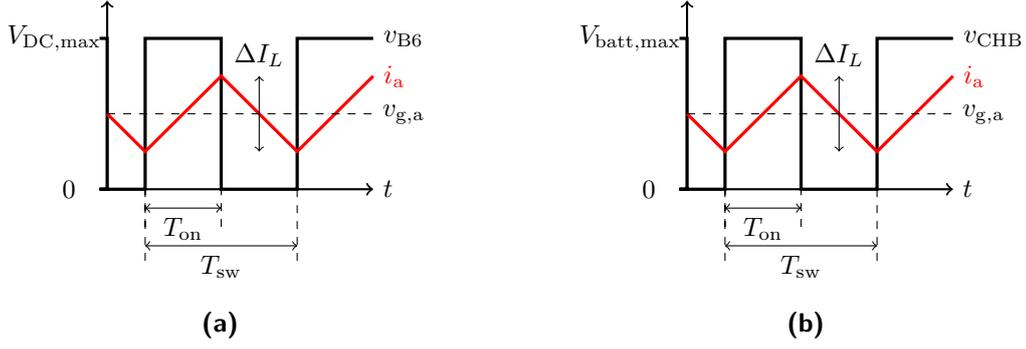
**Figure 7.14** – Inductor's current ripple in case of (a) the B6-bridge and (b) CHB inverter [93].
