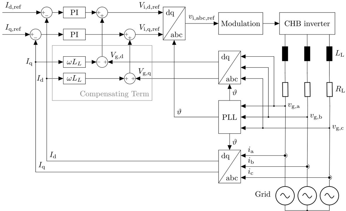
Figure 7.19 – Vector oriented control block diagram [107].
