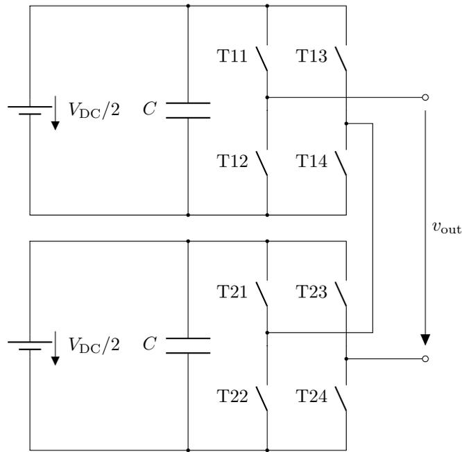
Figure 4.4 – Basic circuit of the CHB inverter.
