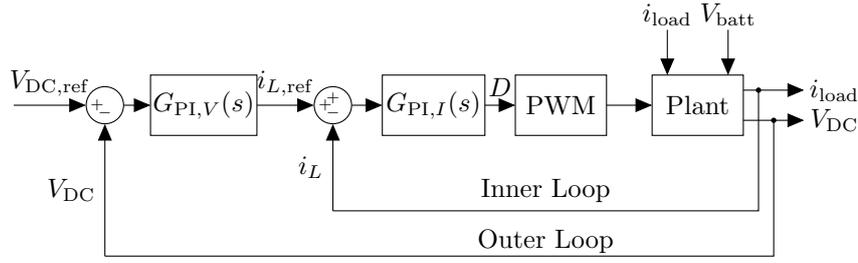
**Figure 5.7** – General cascaded control structure of step-up DC-DC converters [10] [107].
