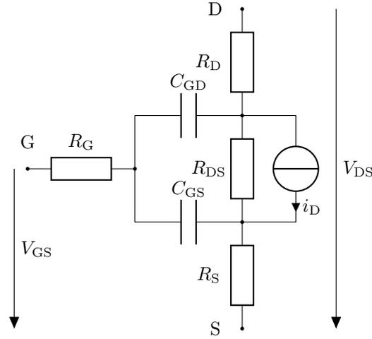
**Figure 6.5** – Circuit diagram used to simulate a MOSFET with the Shichman-Hodges' equations in Simscape.
