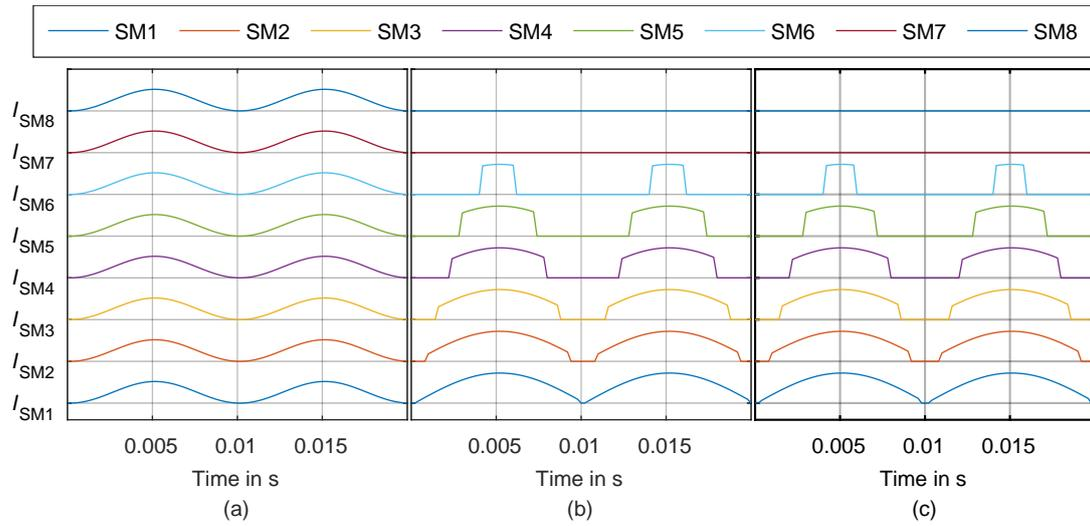
**Figure 8.4** – DC-link current of the submodules of phase a using simulation on system-level using: (a) PSPWM, (b) PD-LSPWM, and (c) NLC.
