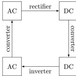
Figure 2.2 – Operation mode of power conversion.
