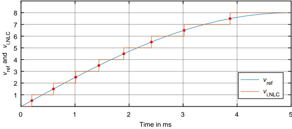
**Figure 7.11** – Output inverter voltage at a given reference signal using NLC.
