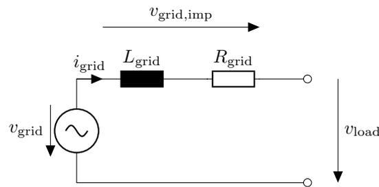
**Figure 2.3** – Grid model to explain the voltage drop over the grid impedance by changing the load.
