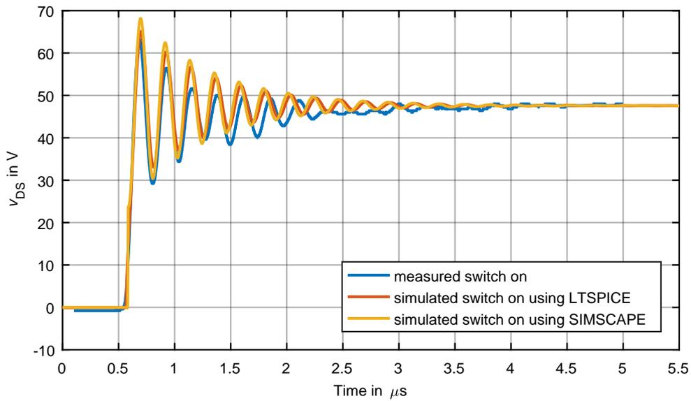
**Figure 6.4** – Drain-source voltage  $V_{DS}$  during MOSFET switch-on time using physical simulations and measurement result [100].
