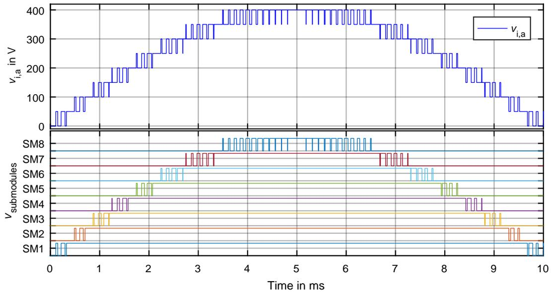
**Figure 7.9** – CHB inverter and submodules voltages using LSPWM.
