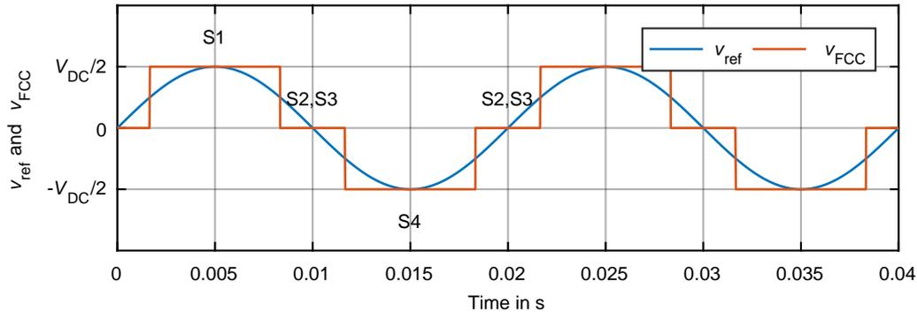
**Figure 4.9** – Output voltage of the circuit in Fig. 4.8 with the switching states in Table 4.4.
