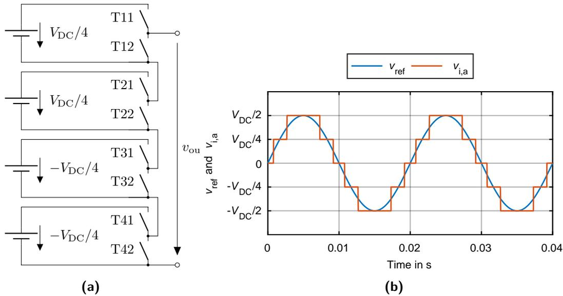
**Figure 4.2** – Schematic circuit for multilevel inverter and its output voltages [183].
