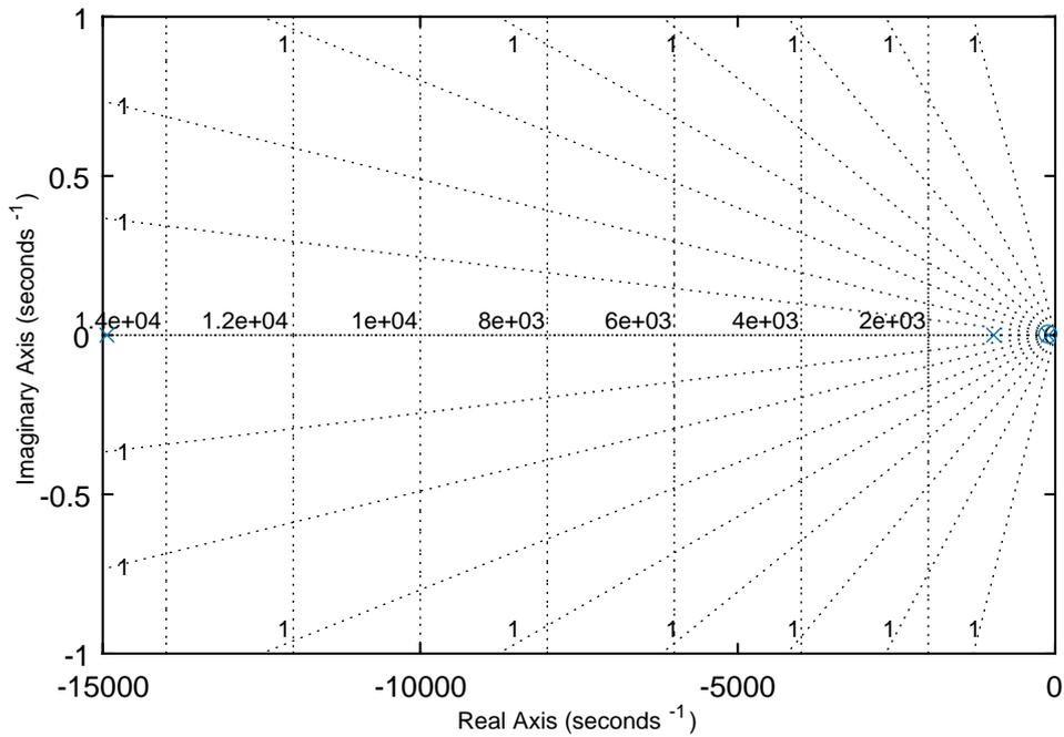
**Figure 7.21** – Pole zero map for the feedback control transfer function  $G(s)_{\text{Plant}}$  of the filter, the inverter, and the PI-controller.
