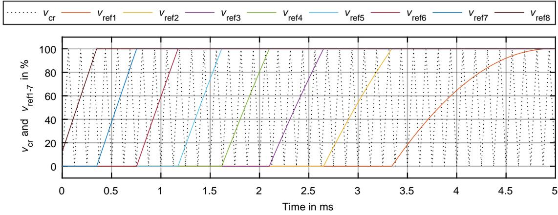
**Figure 7.8** – Reference voltages and carrier-signals for the 17-level CHB inverter using the proposed method to implement POD-LSPWM.
