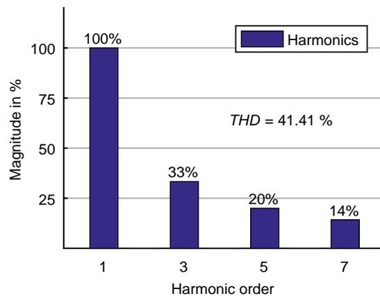
**Figure 2.5** – Harmonic spectrum and  $THD$  of the resulting distorted signal  $v_{dist}$  in Fig. 2.4.
