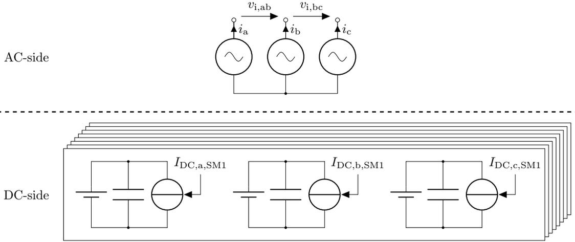
**Figure 8.3** – Average model of the 17-level CHB three-phase inverter on system-level.
