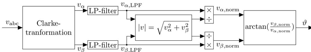
**Figure 7.16** – Low pass transformation angle detector scheme [164].
