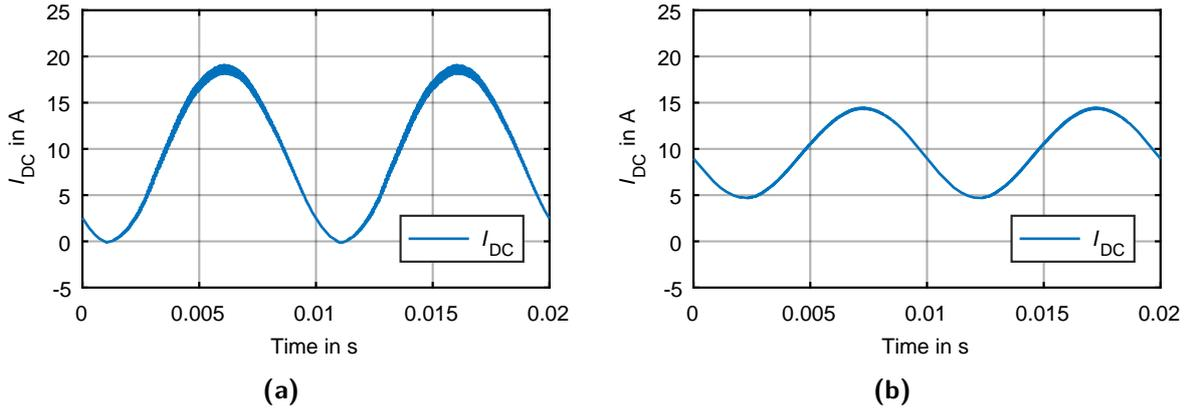
**Figure 3.6** – H-bridge inverter DC-link currents using different capacitance values of (a) 4 mF and (b) 20 mF.
