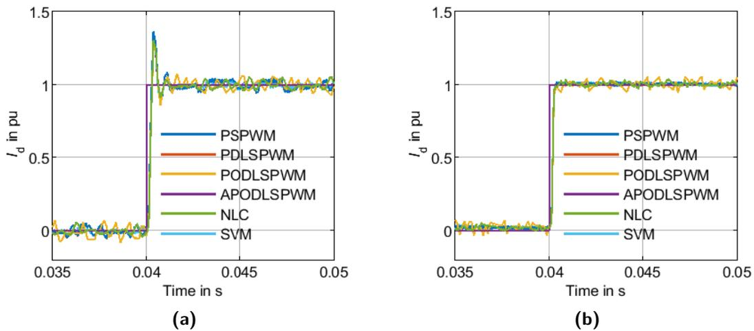
**Figure 7.22** – Step responses using the simulations on circuit-level (a) with and (b) without considering the compensating term.
