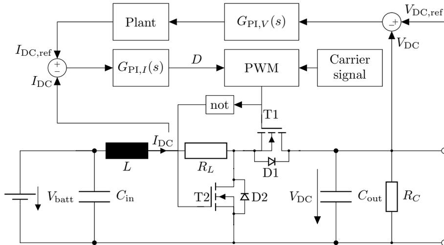
Figure 5.9 – Bidirectional step-up DC-DC converter with cascaded control structure [10].
