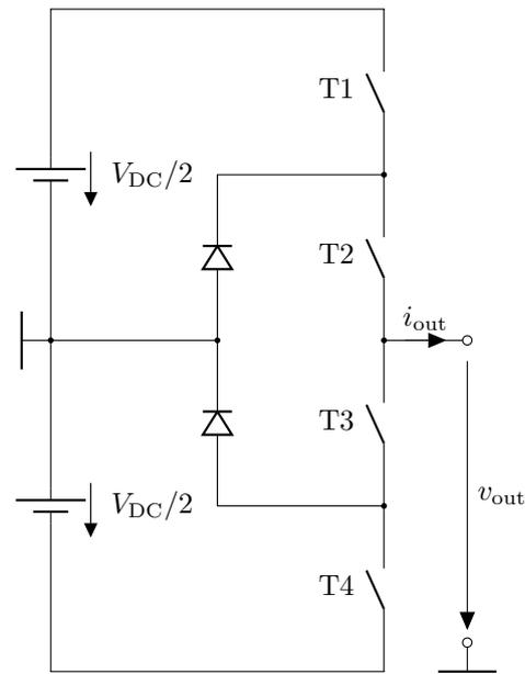
Figure 4.6 – Basic circuit of the neutral point clamped inverter.
