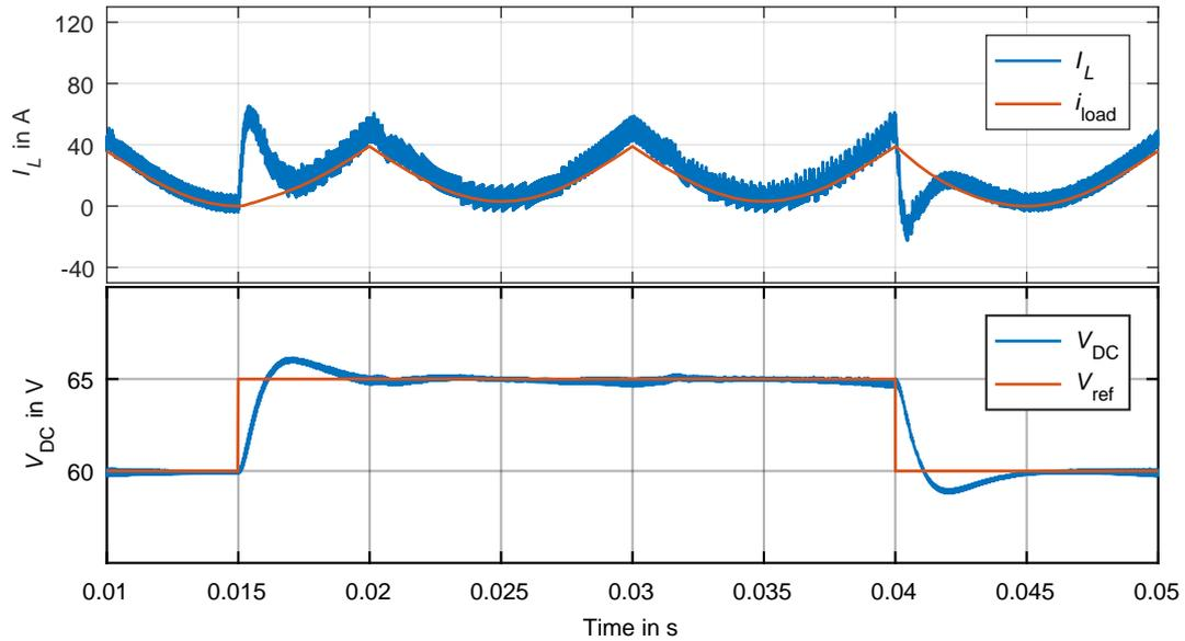
**Figure 5.13** – Step-up DC-DC converter's inductor current  $I_L$  and DC-link voltage  $V_{DC}$  in case of non-linear load with the proposed feed-forward control [107].
