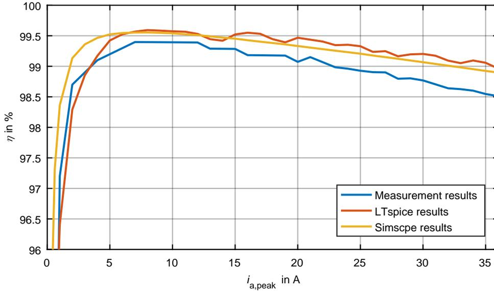
**Figure 6.8** – CHB inverter efficiency considering the power losses in all H-bridge inverters and the power filter used.
