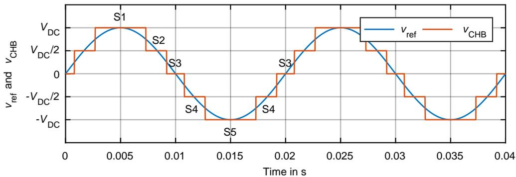
Figure 4.5 – Output voltage of the circuit in Fig. 4.4 with the switching states in Table 4.2.
