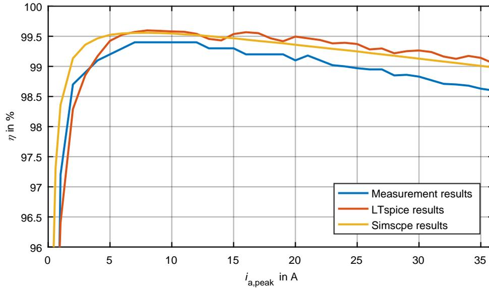
**Figure 6.7** – H-bridge inverter efficiency at different load current using Simscape and LTspice simulations and measurements with power analyzer PA4000 [105].
