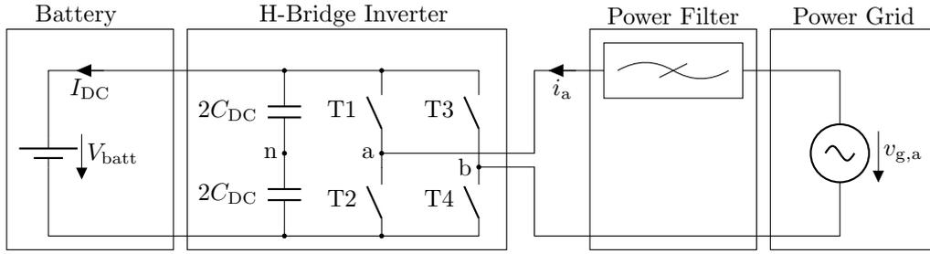
**Figure 3.1** – System overview of conventional H-bridge inverter to be used in single-phase battery energy storage system.
