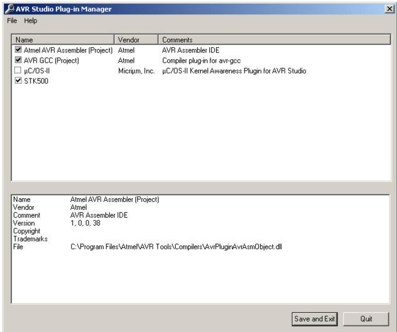
The list shows all the installed plug-ins with name, vendor and comment. All the enabled plug-ins are marked with a checked box. Click on this box to disable (uncheck) or enable (check) the plug-in.
