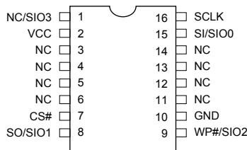
**16-PIN SOP (300mil) for MX25L12845E**
