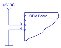
The board can be connected as shown above. Both alternatives are possible and can be used as they fit best into the layout of the carrier board. The two VCC PINs and the two GND PINs are connected internally.
