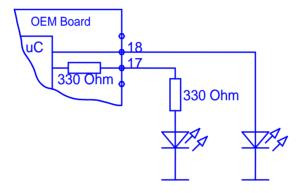
In both cases the LED supply voltage levels are TTL levels.
