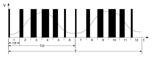
In using not every second sample but every third, fourth, fifth... it is possible to generate Nc different frequencies in the range from [1/T Hz .. 0 Hz]. Note: for high frequencies it will not be a sine wave anymore. The step-width between samples is specified by  $X_{SW}$ . Equation 5 describes this relation:
