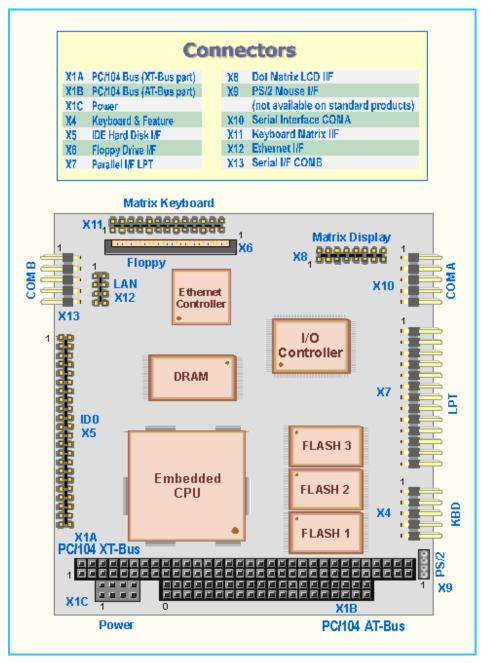
Pin 1 of any connector is marked with a rectangular pad at the bottom side of the board.
