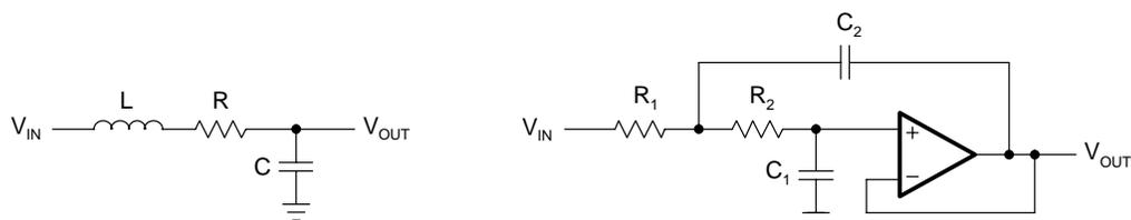
Figure 16–1. Second-Order Passive Low-Pass and Second-Order Active Low-Pass
