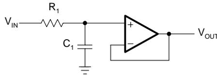
Figure 16–14. First-Order Noninverting Low-Pass Filter with Unity Gain
