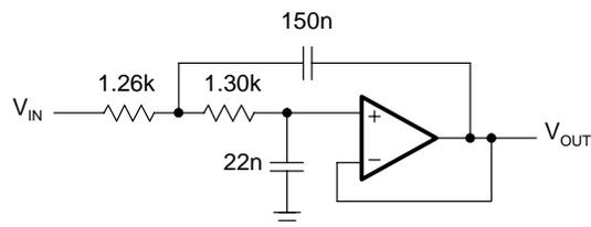
**Figure 16–17. Second-Order Unity-Gain Tschebyscheff Low-Pass with 3-dB Ripple**
