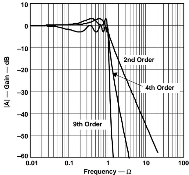
Figure 16–6. Gain Responses of Tschebyscheff Low-Pass Filters
