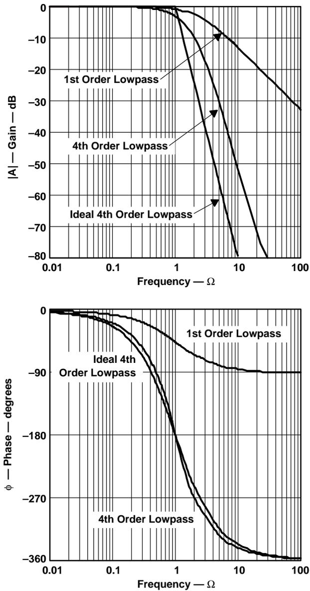
**Note:** Curve 1: 1<sup>st</sup>-order partial low-pass filter, Curve 2: 4<sup>th</sup>-order overall low-pass filter, Curve 3: Ideal 4<sup>th</sup>-order low-pass filter
