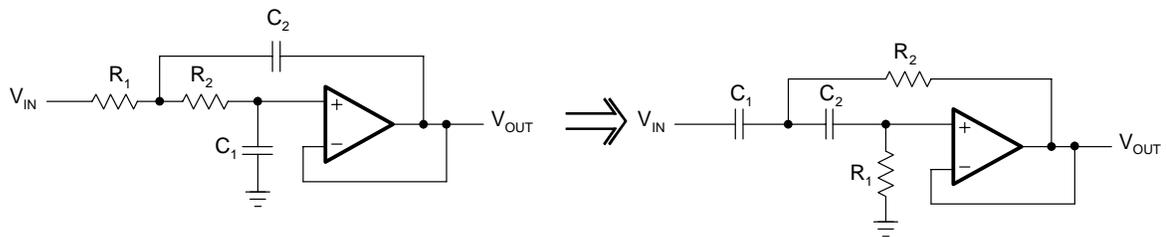
Figure 16–23. Low-Pass to High-Pass Transition Through Components Exchange
