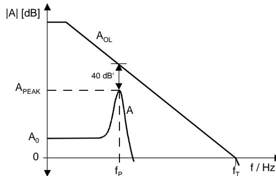
Figure 16–53. Open-Loop Gain ( $A_{OL}$ ) and Filter Response ( $A$ )
