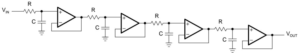
Figure 16–3. Fourth-Order Passive RC Low-Pass with Decoupling Amplifiers
