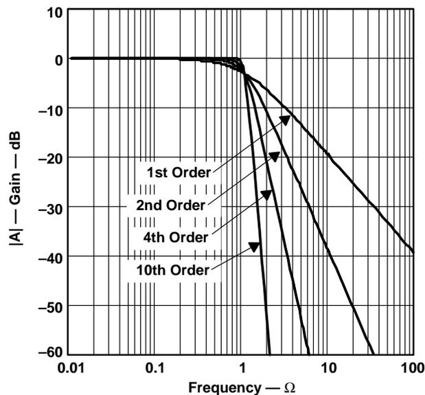
Figure 16–5. Amplitude Responses of Butterworth Low-Pass Filters
