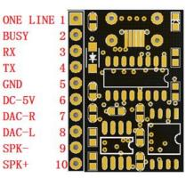
Labels Pins Descriptions 1 ONE LINE One-line interface port BUSY HIGH when playing, LOW in other conditions 2 Data receive port; to be connected with TX of MCU RX 3 4 ТΧ Data transmit port; to be connected with RX of MCU 5 GND Ground 6 DC-5V Power supply; 3.3V - 5.0V 7 DAC-R DAC right channel audio out 8 DAC-L DAC left channel audio out 9 SPK -To Speaker 10 SPK + To Speaker
