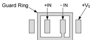
Figure 1. Use a guard ring around sensitive pins
