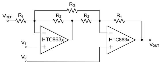
$$V_{OUT} = (V_1 - V_2) \left( 1 + \frac{R_1}{R_2} + \frac{2R_1}{R_G} \right) + V_{REF}$$
