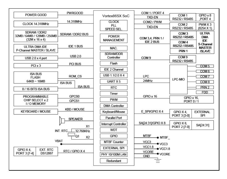
GPIO port 0,1 and 2 are always free for use normally. If your system does not use external RTC and SPI, GPIO port 3 is also free for use. Developer also can disable COM1 to select GPIO port 4. The actual free GPIO pins depend on your system. Please check it before using GPIO.
